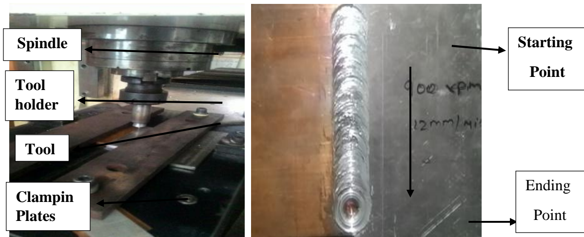
Fig 3.2 Fig shows the experimental setup and welded joint
