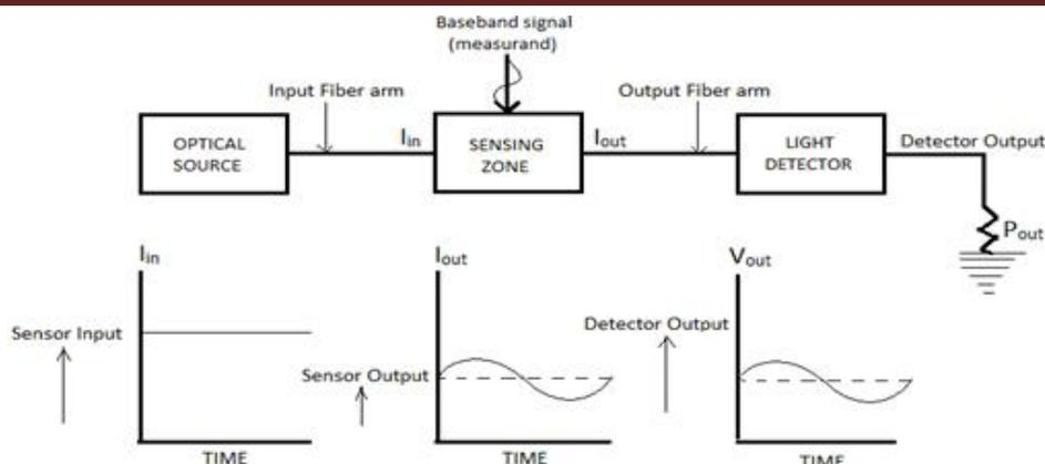
**Fig. 1:** General configuration of an intensity modulated sensor
