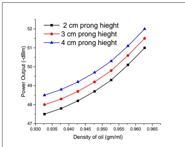
**Fig. 3:** Density versus Output Power when 2 cm/ 3 cm/ 4 cm prong height with 1.5 cm curvature glass rod exposed in oil
