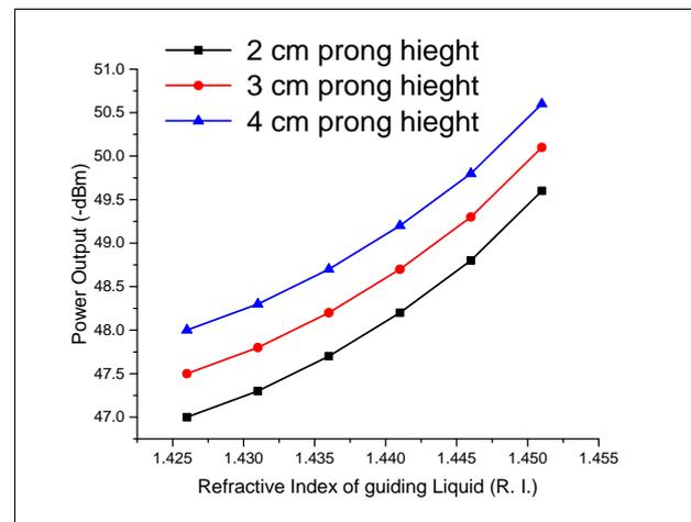
**Fig. 4:** Refractive index of guiding liquid versus Output power when 2 cm/ 3 cm/ 4 cm prong heights exposed to 25 ml oil.
