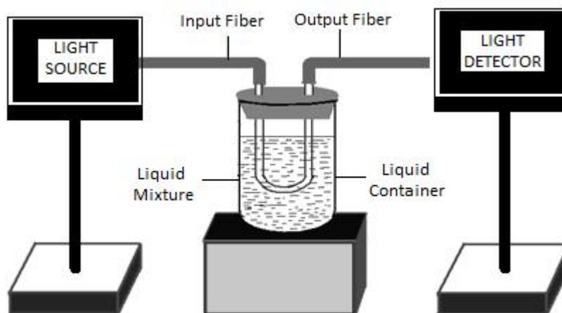
**Fig. 2:** Experimental arrangement of sensor
