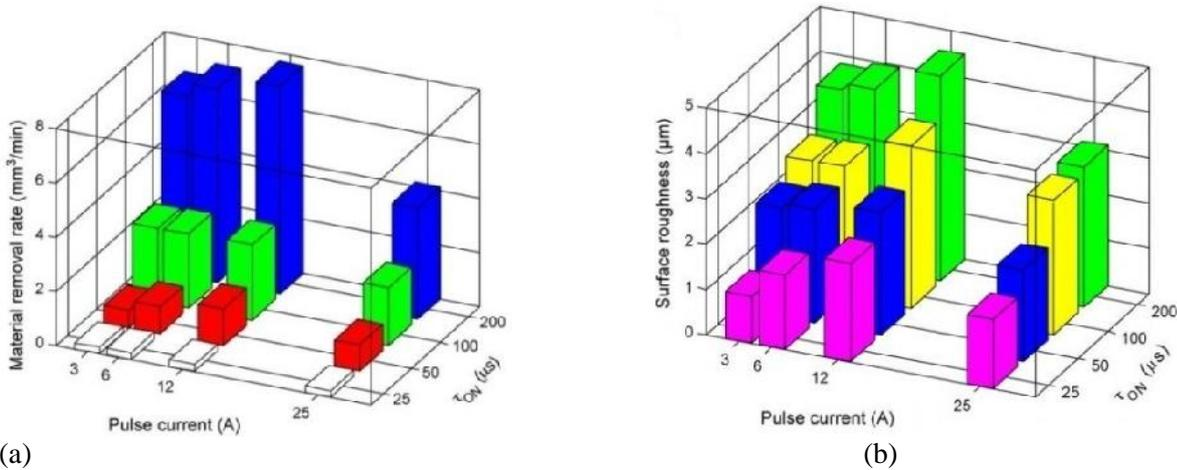
**Fig.7. Effect of Al electrode on (a) MRR and (b) SR[15]**
