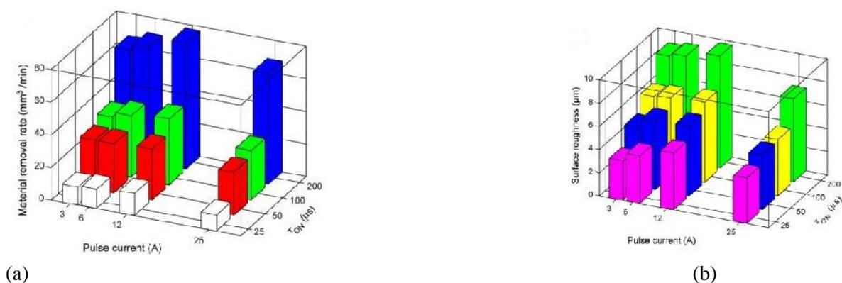
**Fig.4 Effect of (a) MRR and (b) SR with graphite electrode in kerosene [15]**
