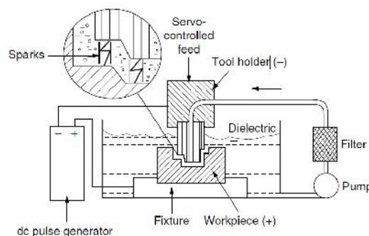
**Fig.1 Schematic diagram of EDM [1]**
