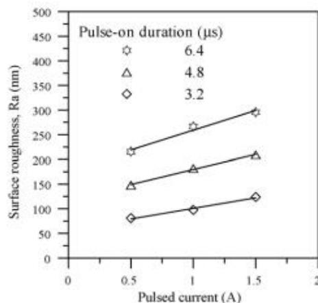
**Fig.3. The average surface roughness at various machining conditions. [13]**
