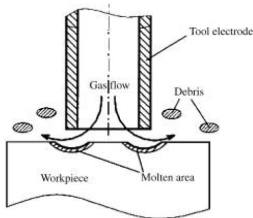
**Fig.2 Principle of EDM [6]**
