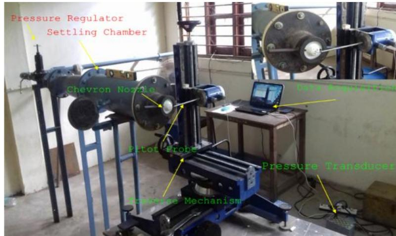
**Fig 2.2: Open jet facility setup**
