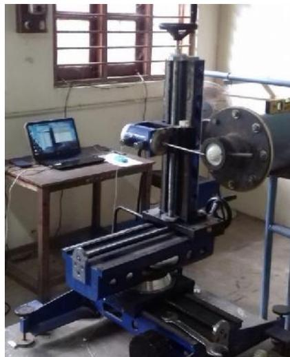
**Fig 2.3: Traverse mechanism**
