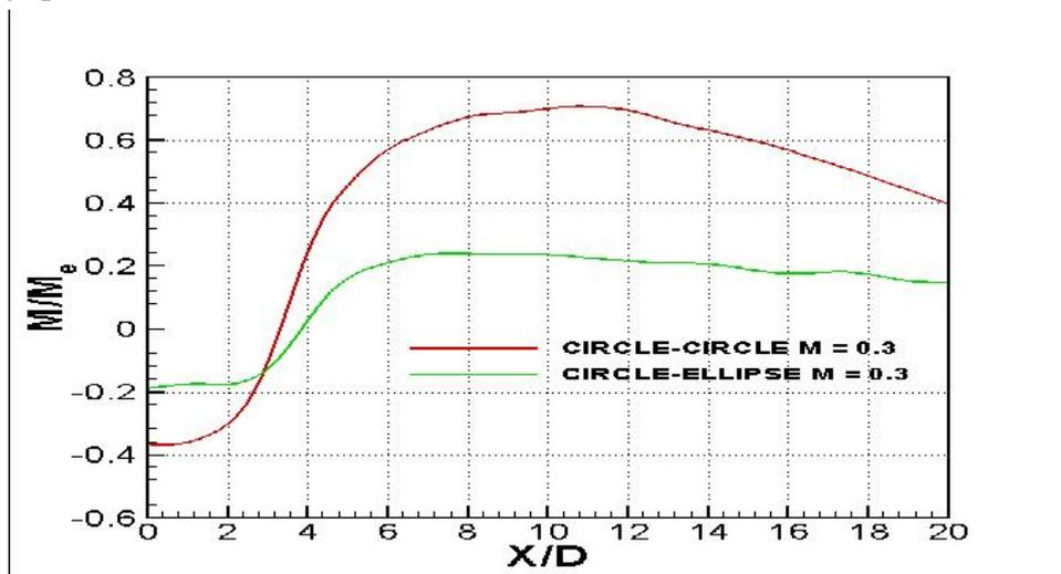
**Fig. 3: centerline Mach number decay of the two twinjets for M = 0.3**
