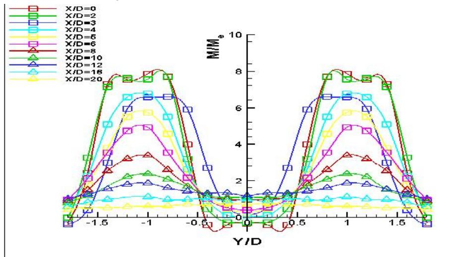
**Fig. 6: radial Mach number decay of the circle-circle twinjet nozzle for  $M = 0.3$**
