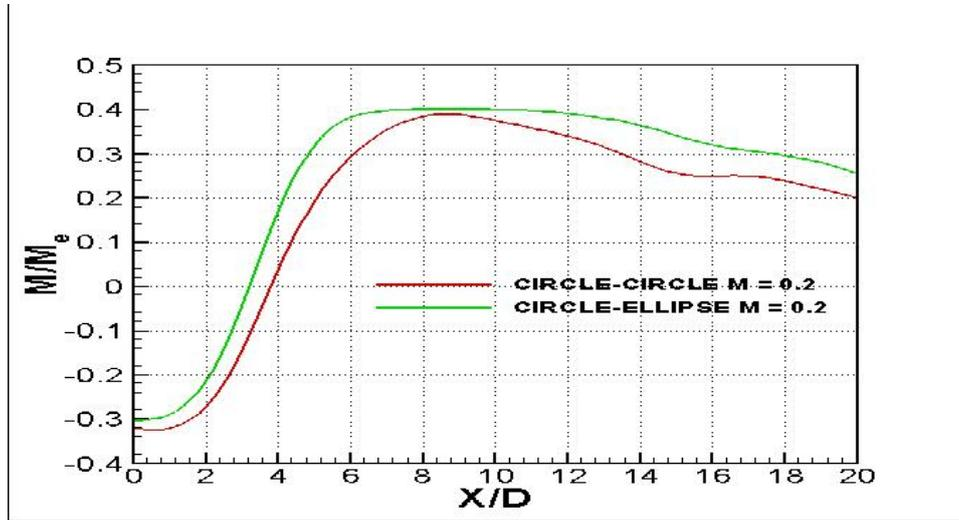
**Fig. 2: centerline Mach number decay of the two twinjets for M = 0.2**
