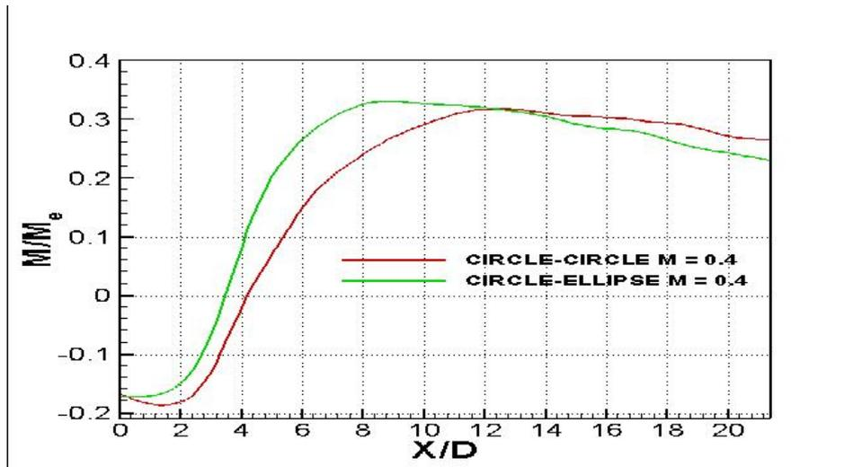
**Fig. 4: centerline Mach number decay of the two twinjets for  $M = 0.4$**
