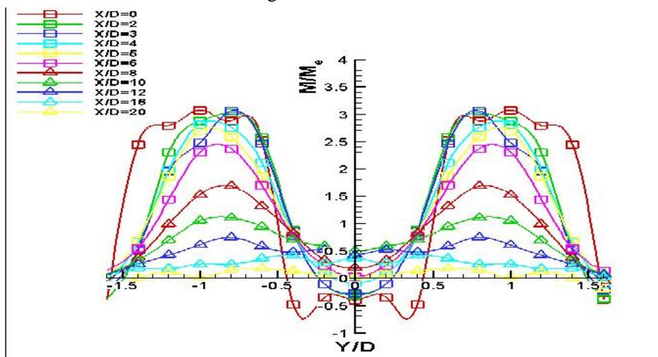
**Fig. 5: radial Mach number decay of the circle-circle twinjet nozzle for  $M = 0.2$**
