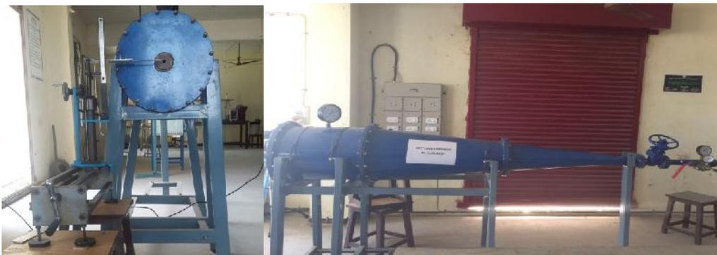
Fig2: Open Jet facility with transverse mechanism and side view
