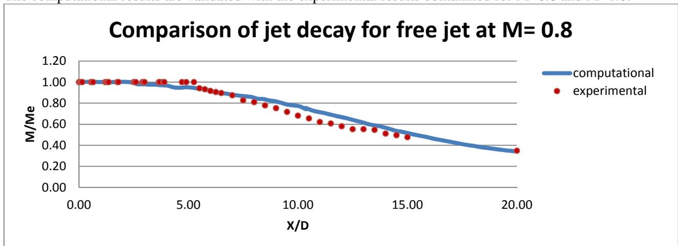
Plot:4 Comparison of jet decay for free jet at  $M=0.8$
