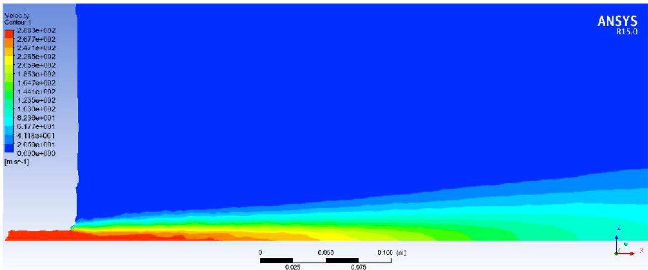
**Fig. 3 Axial velocity magnitude contour for free jet at Mach number 0.8**
