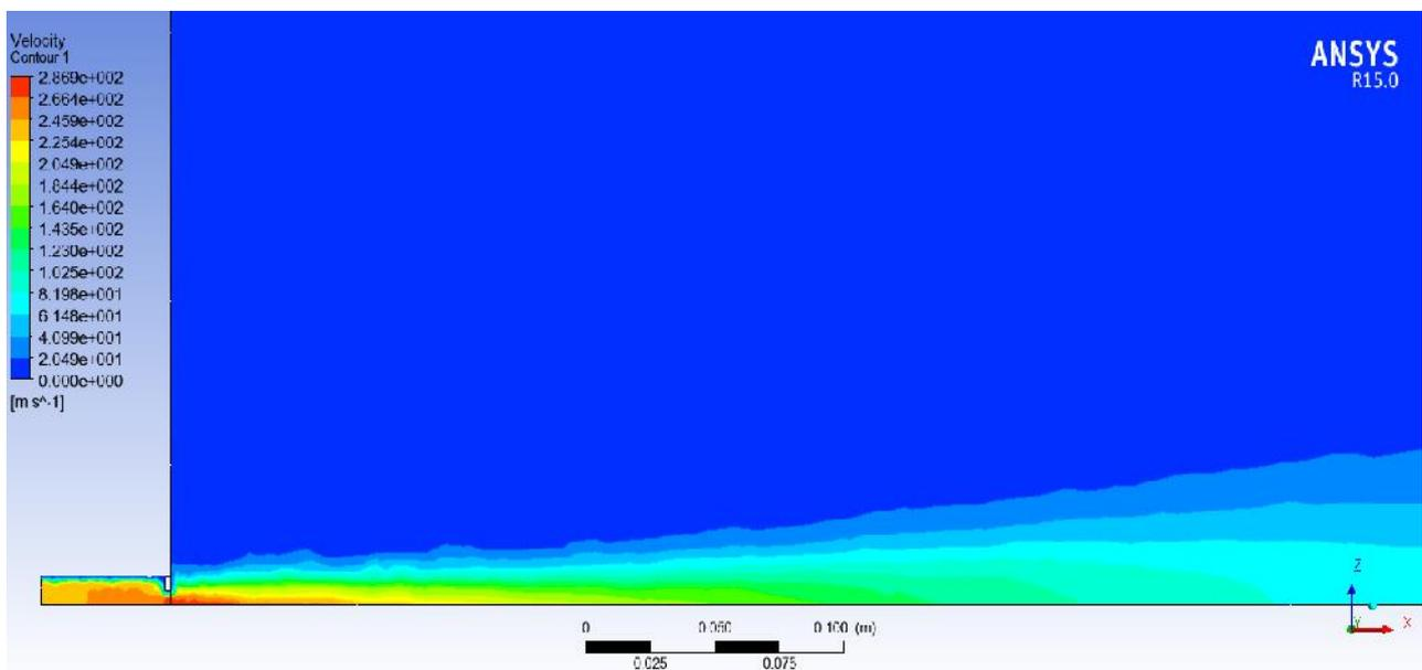
**Fig. 4 Axial velocity magnitude contour for single tab at Mach number 0.8**
