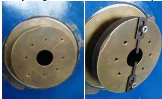
Fig1: Nozzle with and without tabs
