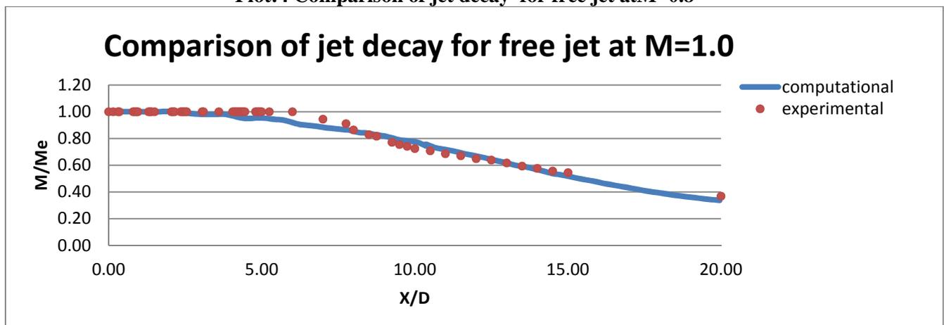
Plot:5 Comparison of jet decay for free jet at  $M=1.0$
