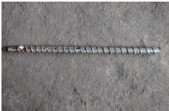
Fig.2: Photograph of failed reciprocating screw.
