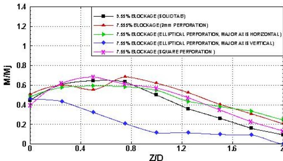
Figure 12. Z- Mach profiles for controlled jets at X/D = 7, M<sub>j</sub> = 0.5
