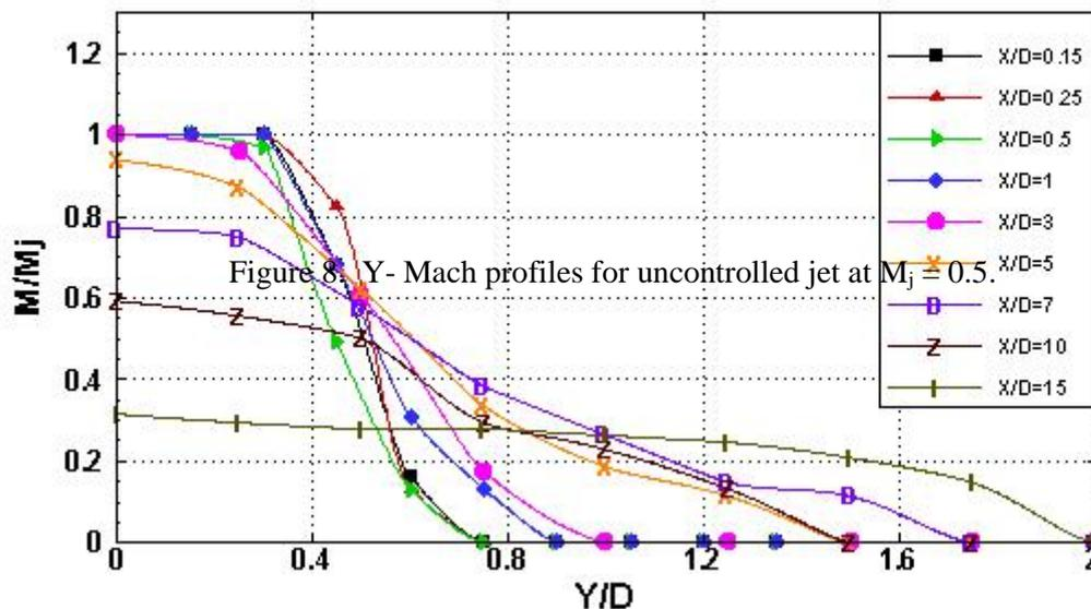
Figure 8. Y- Mach profiles for uncontrolled jet at  $M_j = 0.5$ .
