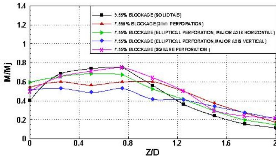
Figure 13. Z- Mach profiles for controlled jets at  $X/D = 1$ ,  $M_j = 0.9$
