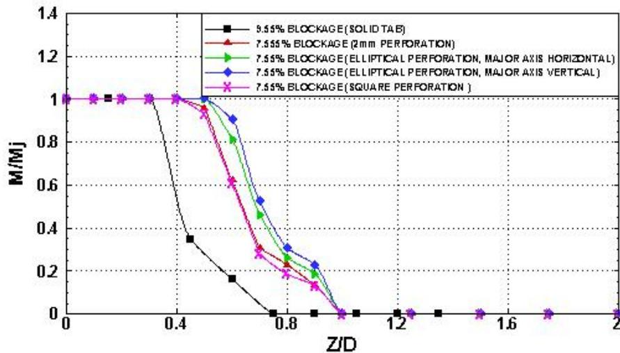
Figure 11. Z- Mach profiles for controlled jets at X/D = 1, M<sub>j</sub> = 0.5
