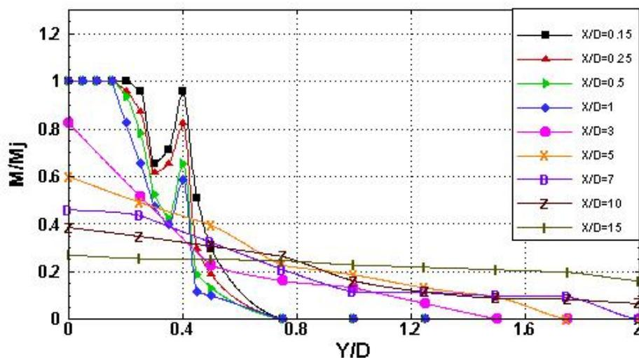
Figure 10. Y- Mach profiles along the tab for elliptical perforation, major axis vertical at different axial locations,  $M_j = 0.5$
