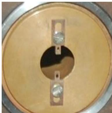
Figure 2. A view of tab arrangement at nozzle exit.
