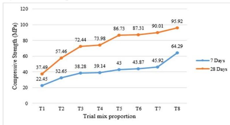
**Fig 1. Compressive strength for trial mix proportions**
