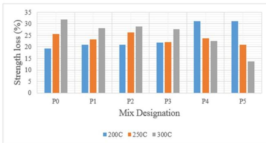
**Fig 5. Percentage weight loss in fire resistance test**
