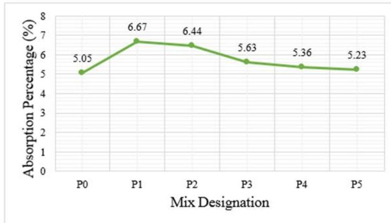
**Fig 4. Water absorption test results**
