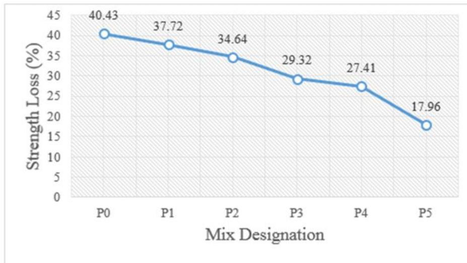
**Fig 7. Strength loss in sulphate resistance test**
