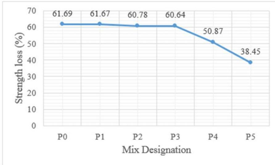
**Fig 6. Strength loss in acid attack test**
