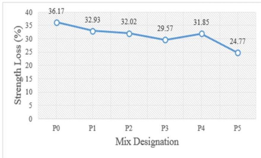
**Fig 8. Strength loss in alkaline attack test**
