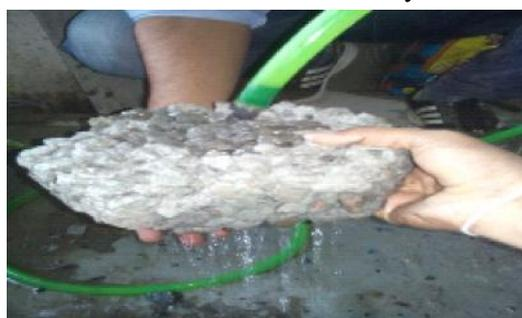
**Fig.8 Permeable paver**
