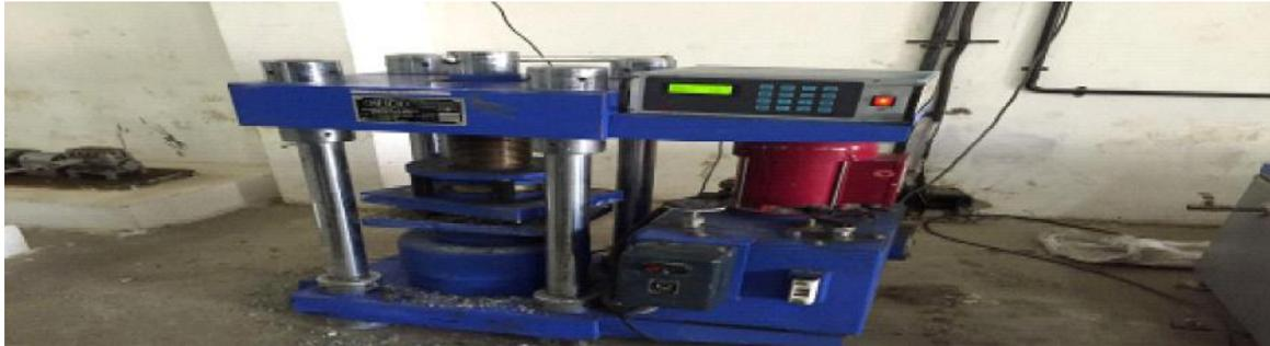
**Fig.4 Compressive testing machine**
