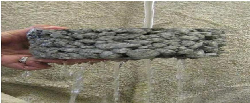
**Fig.1 Pervious concrete**
