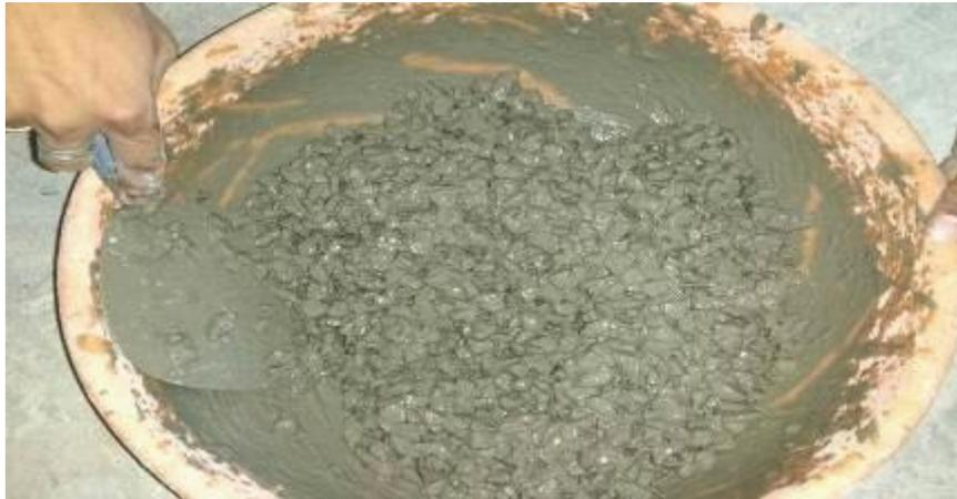
**Fig.9 Pervious concrete mix**
