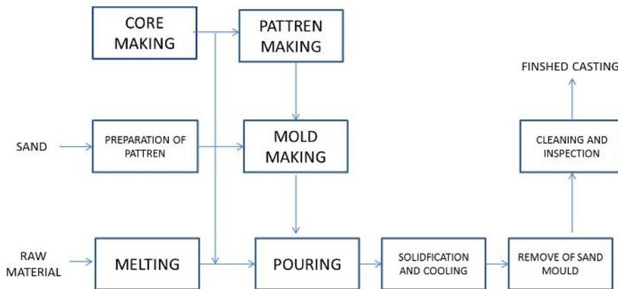
Figure: 4.1 casting process flow line
