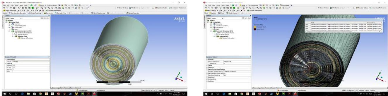
Fig 7: Model of stack imported in ANSYS© and meshed view of stack (with errors)
