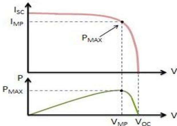
Fig.2. P-V and I-V curve of a solar cell at a particular temperature & irradiation
