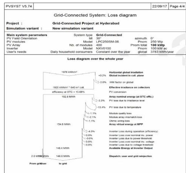
Fig.4 Loss diagram over the entire year
