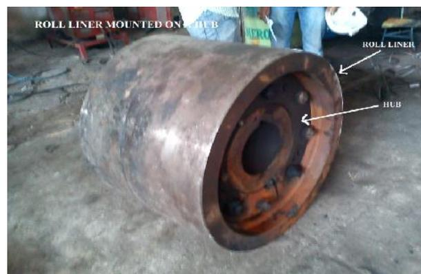
**Figure1 Roll Liner mounted on its hub**
