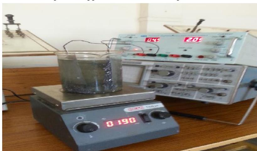
Figure 3: Experimental representation of Electro-Coagulation
