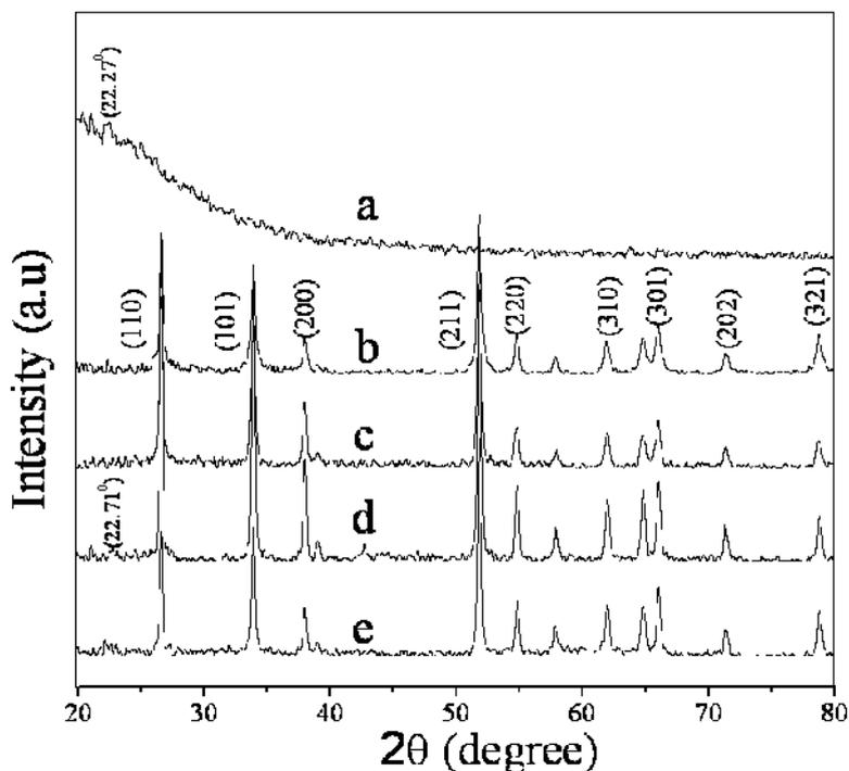
**Figure 1 (a-c)** XRD patterns of (a)  $\text{SiO}_2$  (b)  $\text{SnO}_2$  and (c) 10 wt %  $\text{SnO}_2/\text{SiO}_2$  (d) 15 wt %  $\text{SnO}_2/\text{SiO}_2$  (e) 20 wt %  $\text{SnO}_2/\text{SiO}_2$
