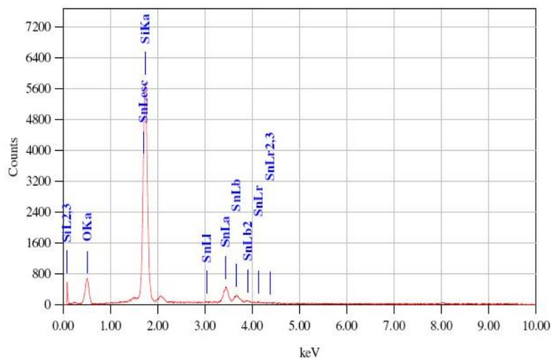
**Figure 4** EDS pattern of 15 wt % SnO<sub>2</sub>/SiO<sub>2</sub>
