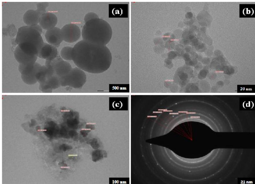
**Figure 2 (a-d)** TEM image of (a) SiO<sub>2</sub> (b) SnO<sub>2</sub> (c) 15 wt % SnO<sub>2</sub>/SiO<sub>2</sub> (d) diffraction patterns of SnO<sub>2</sub>
