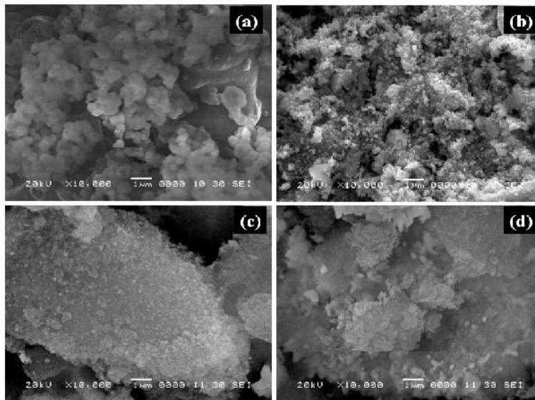
**Figure 3** (a-c) SEM image of (a) SiO<sub>2</sub> (b) SnO<sub>2</sub> (c-d) 15 wt % SnO<sub>2</sub>/SiO<sub>2</sub>
