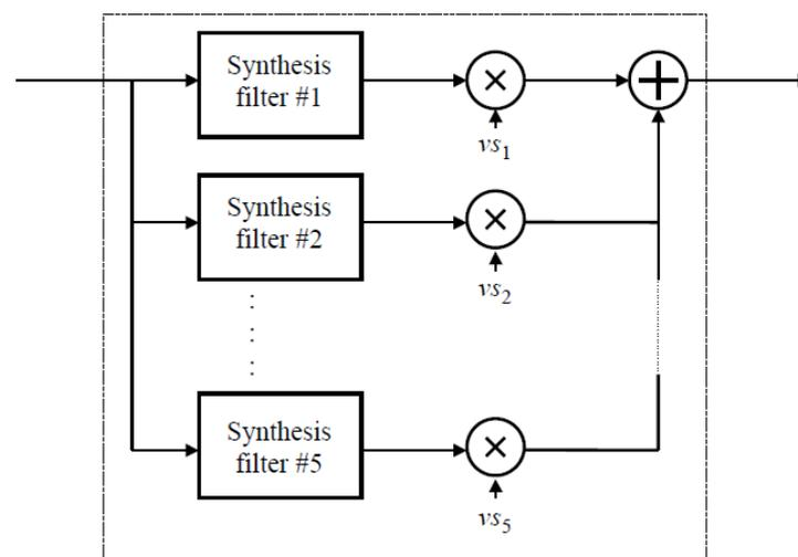
**Figure 2: Block diagram of the pulse shaping filter**
