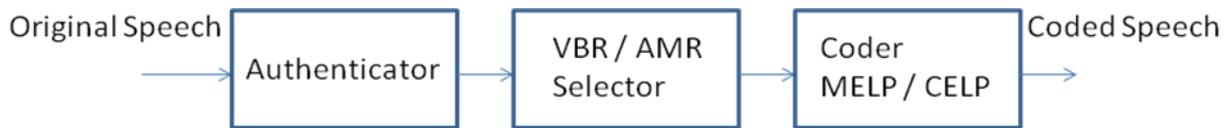
**Figure 3 Block diagram of encoder**
