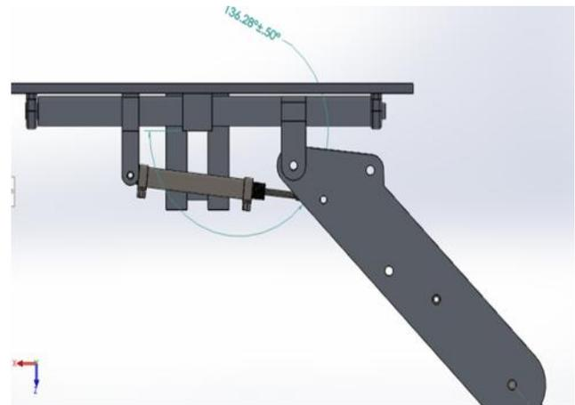
Figure 3: Range of actuation of Thigh piston.
