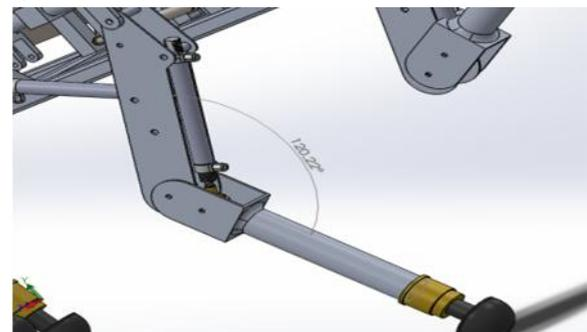
Figure 4: Range of actuation of Knee piston.
