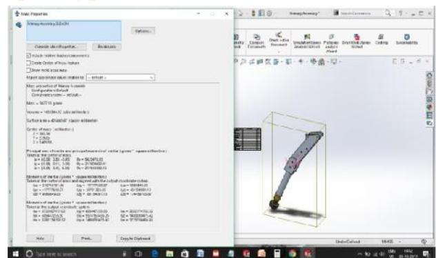
Figure 11: Mass of Leg Assembly. On the right, the Moments of Inertia are listed out.
