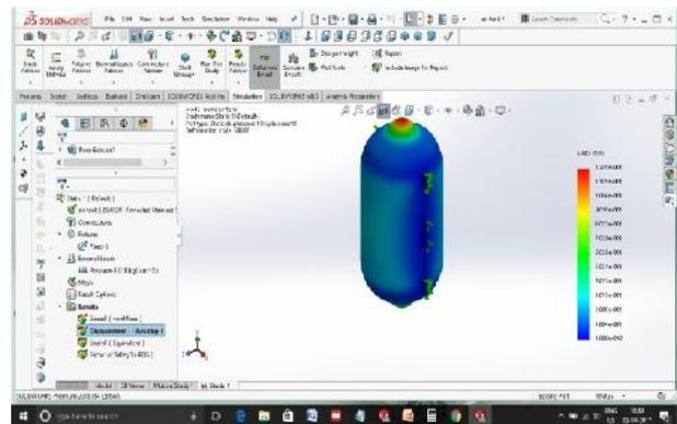
Figure 13: Displacements incurred by pressure vessel due to internal pressure of 10 bar(Operating Pressure).
