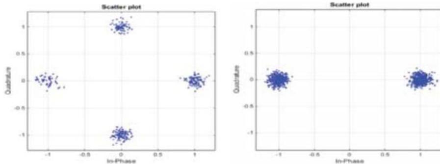
**Figure 5: BPSK and QPSK Constellation for primary user signal.**
