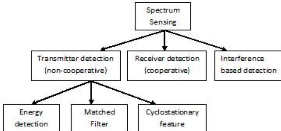
**Figure 1: Various spectrum sensing techniques**
