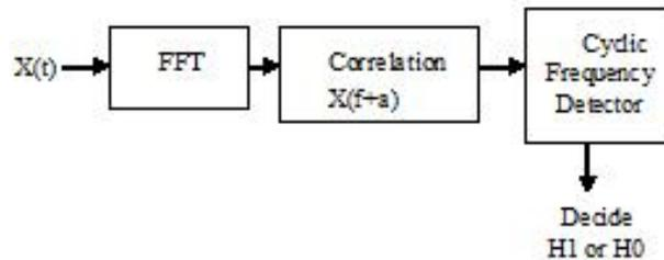
**Figure 4: Cyclostationary detection**
