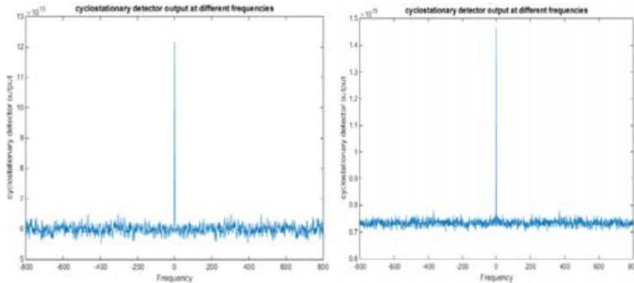
**Figure 8: Cyclostationary detector output for low SNR values.**
