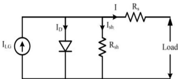
Fig 2: Model of a PV Cell.
