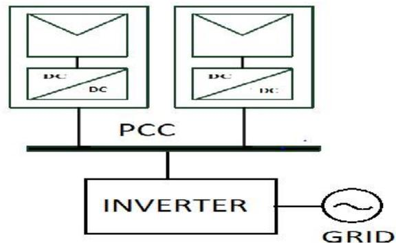
Fig:3 Micro Inverter based grid connected PV system.
