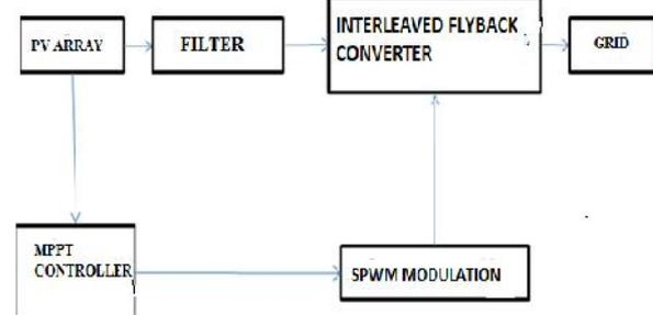
Fig.1 Block diagram of grid-tie PV power system with interleaved flyback converter.
