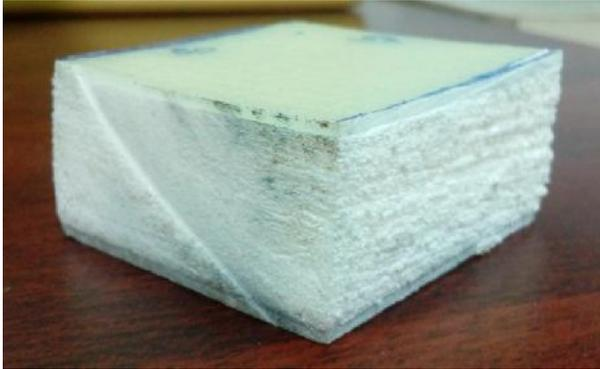
**Fig 2: A- Sandwich, Thickness = 39mm**
