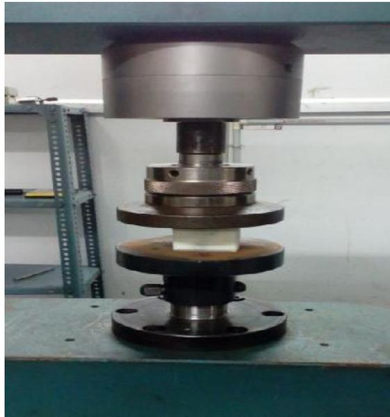
Fig 8: Flatwise Compression Test set up
