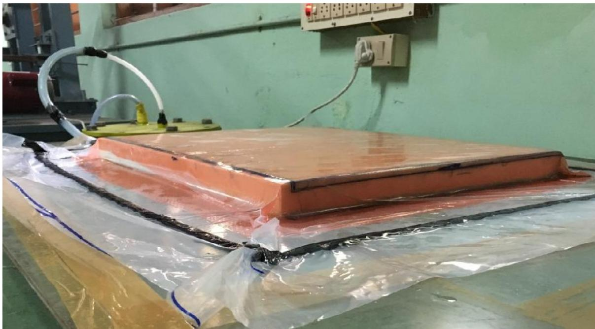
**Fig 1: Fabrication of Sandwich by Vacuum Bag Molding Process**
