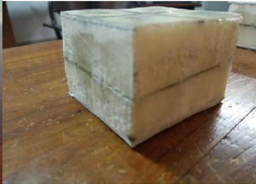
**Fig 3: C- Sandwich, Thickness = 40mm**
