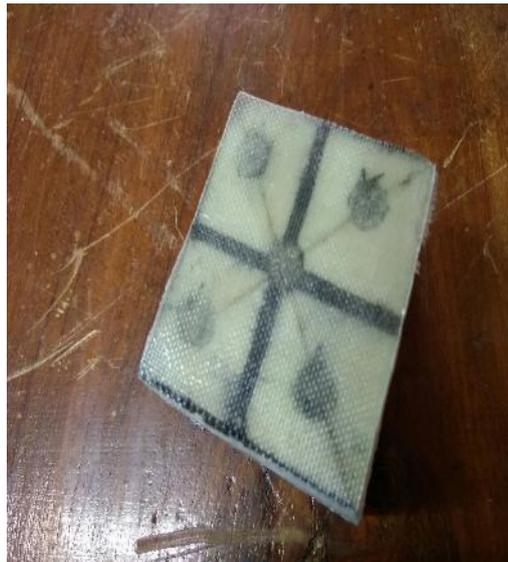
**Fig 7: Fabricated Sandwich with grooves
