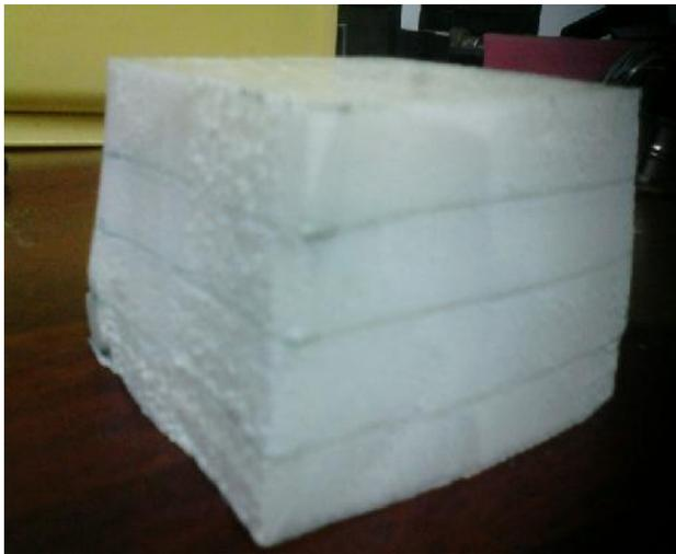
**Fig4: Multilayer Sandwich, Thickness=42mm**
