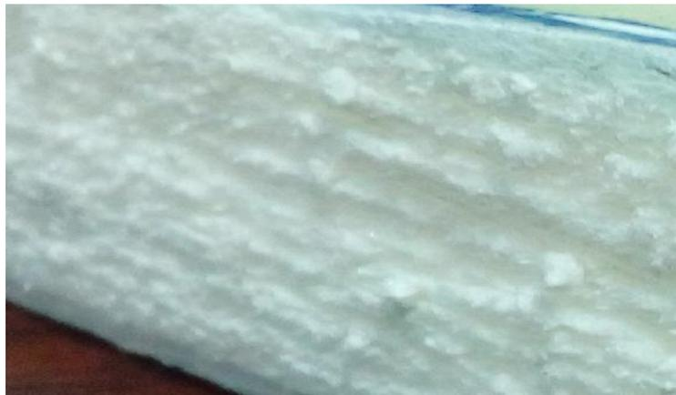
**Fig 9: Bulging/Densification of Core**
