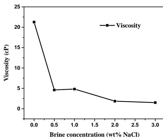
**FIG 2: Effect of NaCl concentration on viscosity of the  $C_{16}mimBr-NaSal$  solution (14mM each)**
