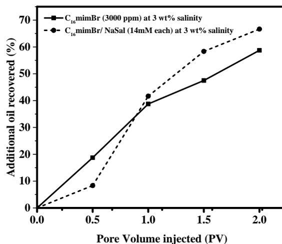
**FIG 5: Additional oil recovered during surfactant flooding**
