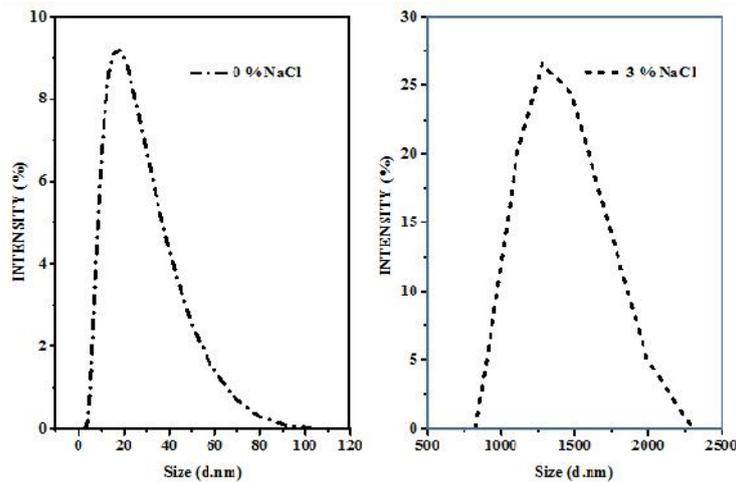
**Fig 4: Influence of change in NaCl concentration on the size of emulsion formed in the homogenized solution of  $C_{16}mimBr$ -NaSal and oil**
