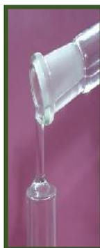
**Fig 1: Pictorial representation of highly viscous surfactant formulation prepared on mixing of  $\text{C}_{16}\text{mimBr}$  ~ 14 mM and  $\text{NaSal}$  ~ 14 mM in distilled water.**
