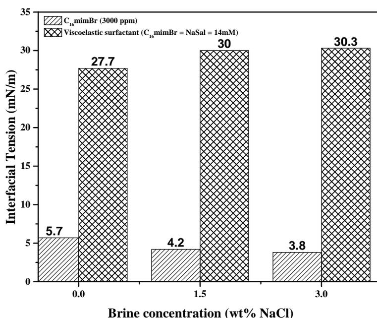
**Fig 3: Effect of NaCl concentration on IFT between  $C_{16}mimBr$  /oil solution as well as  $C_{16}mimBr-NaSal$ / oil solution.**
