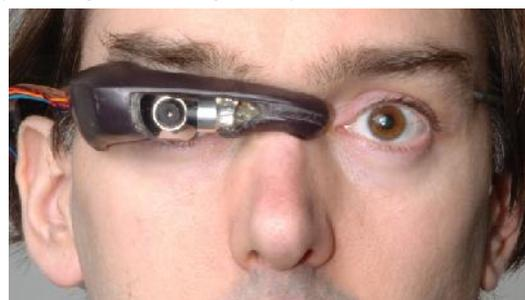
**Fig.5: Eyetap model of Augmented Reality**
