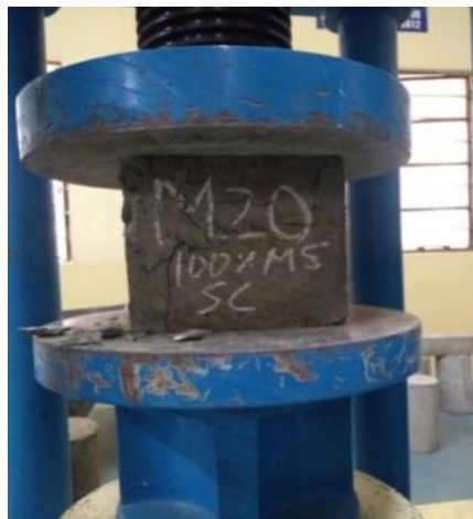
Fig 2: cube specimen testing
