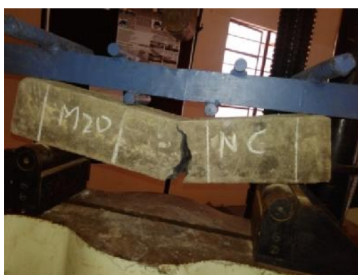
Fig 3: Beam specimen testing
