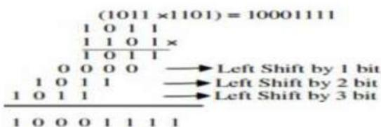
Fig.1: Example of conventional multiplier
