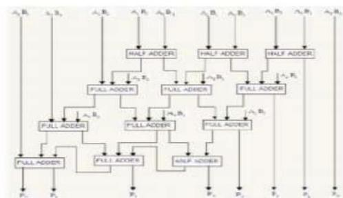
Fig.3: Structure for conventional multiplier
