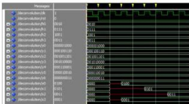
Fig.6: Simulation results of Deconvolution using Vedic mathematics
