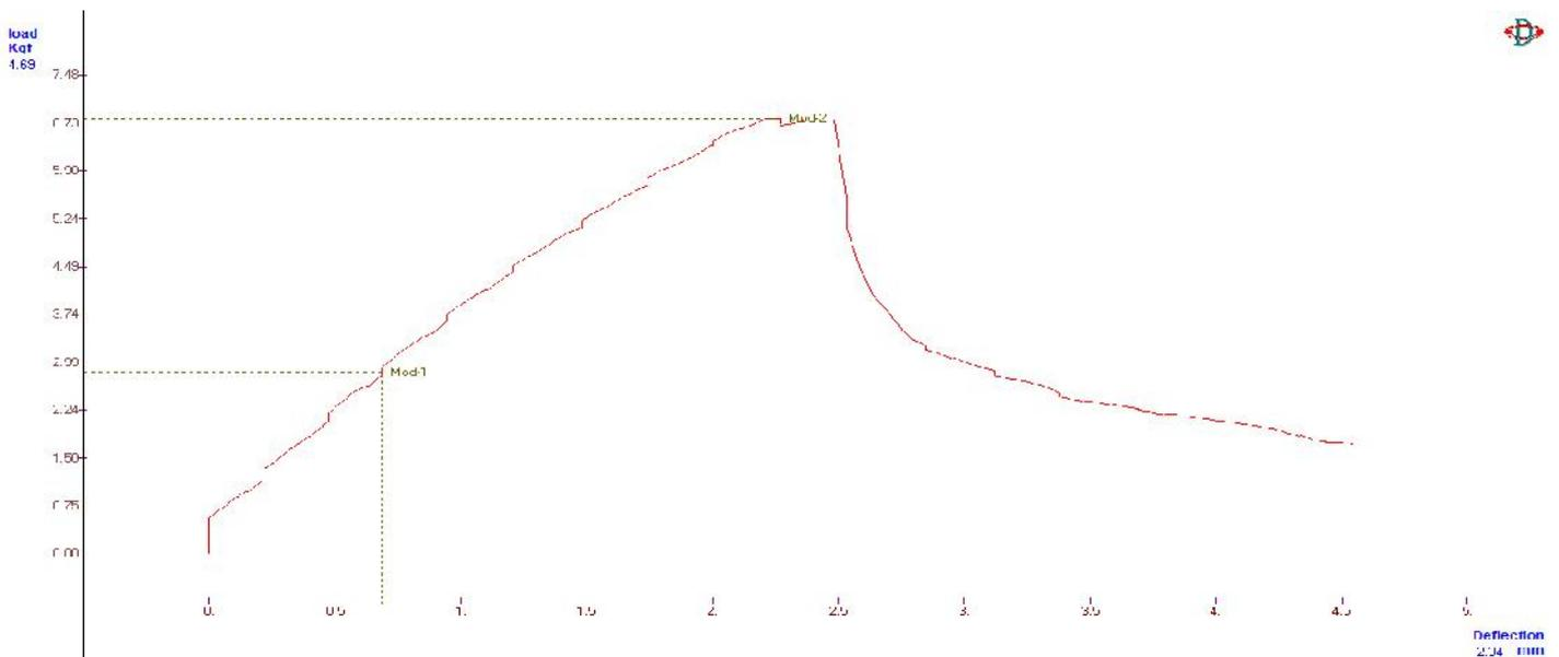
Fig.15 Flexural Test for untreated Caryota Urens :Deflection vs Load
