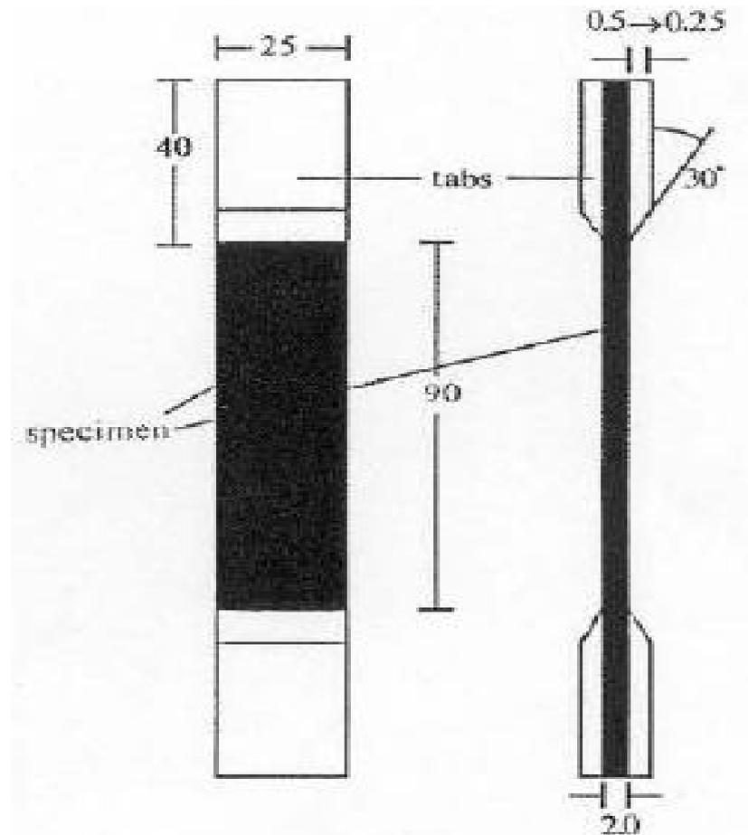
Fig. 11 Typical tensile composite test specimen (all dimensions in mm)
