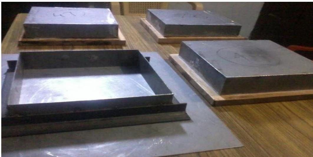
Fig.5 Fabrication of Die
