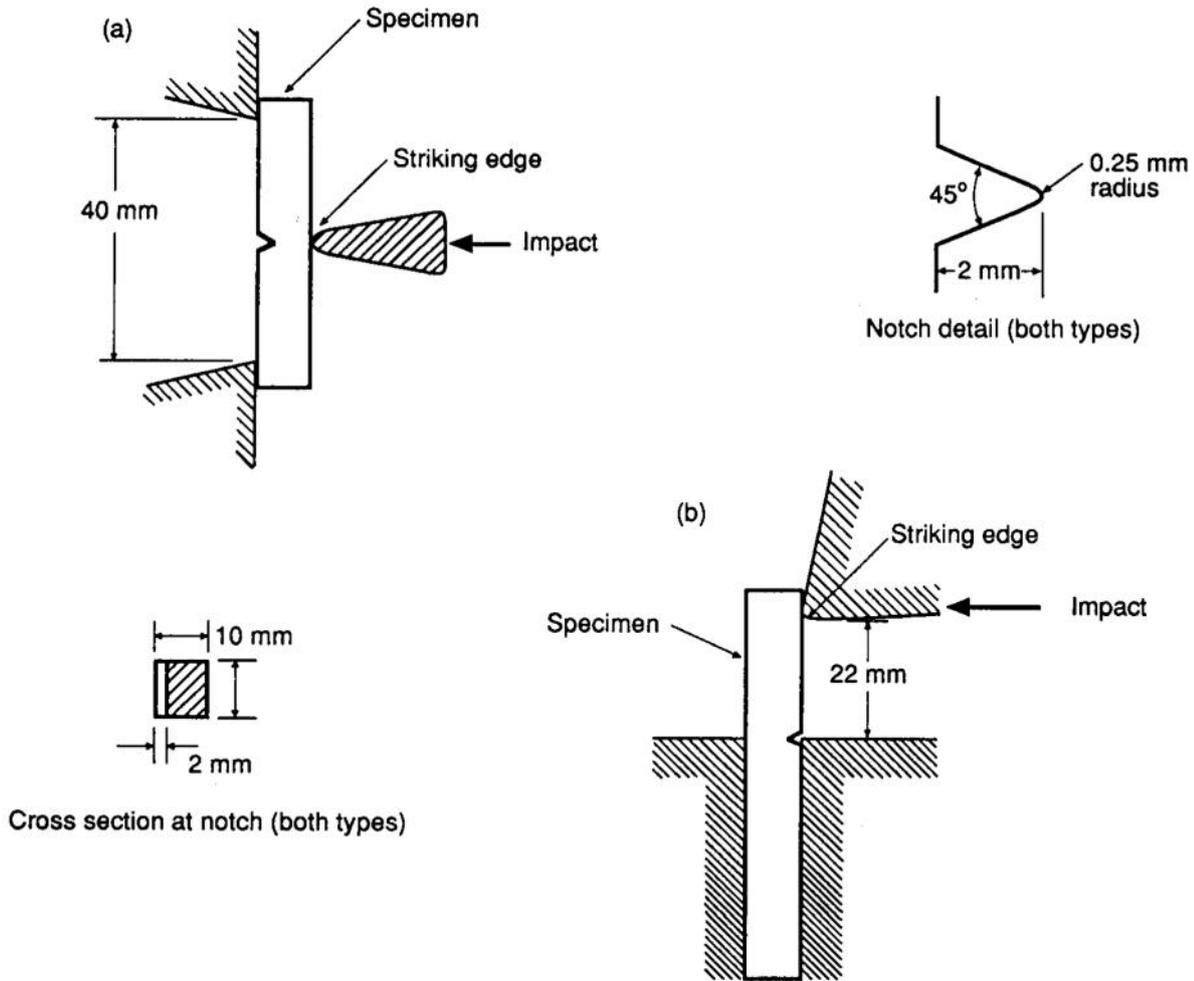
Fig.9 Impact Test Specimen
