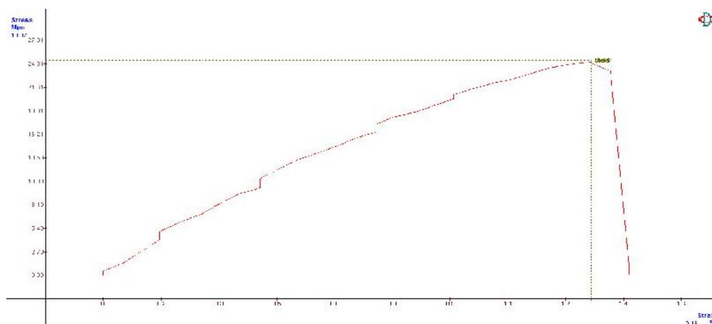
Fig.17 Tensile Test for untreated Caryota Urens : Strain vs Stress
