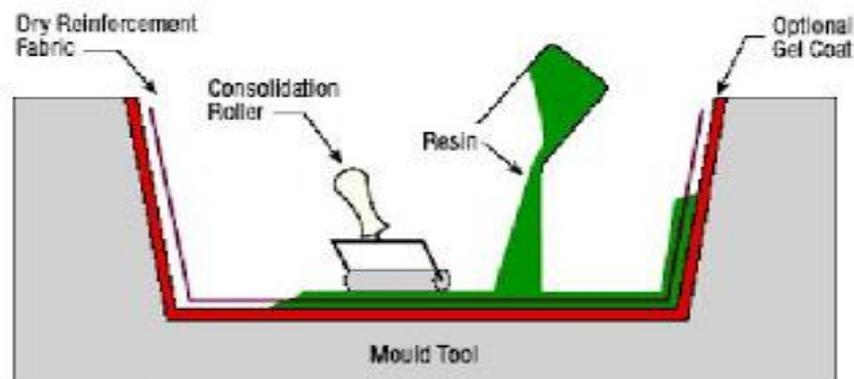
**Fig.6 Hand layup / Wet layup process**
