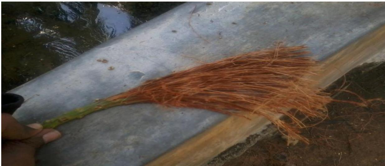
Fig.4 Beating process was carried out for extracting the fiber from caryota urens.
