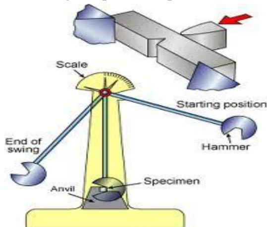
Fig.10 Impact Testing
