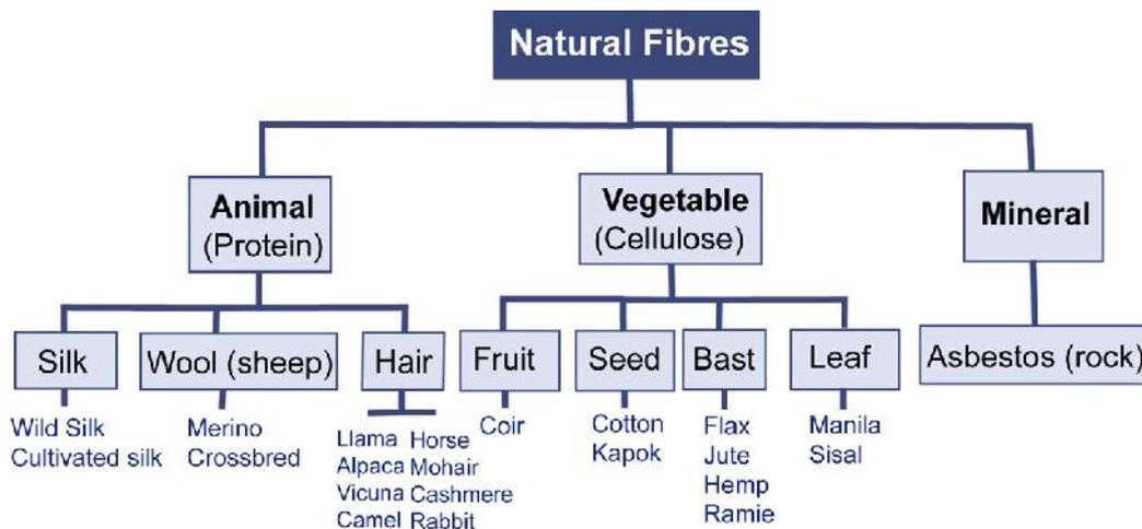
Fig. 1 Classification of natural fibers which can be used as reinforcement of Polymer.
