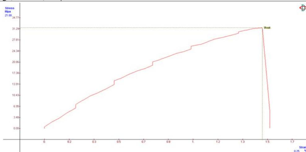
Fig.16 Tensile Test for treated Caryota Urens : Strain vs Stress
