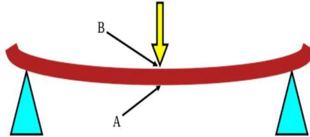
Fig.13 Flexural test with three point load
