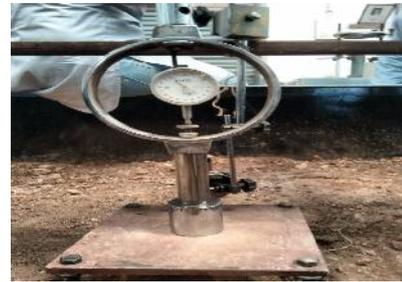
**Fig.3** Sensitive Dial Gauge for Recording Settlement
