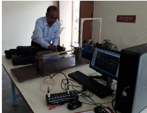
Figure 3.1 Experimental Setup of FFT analyzer
