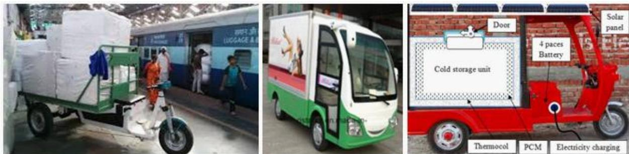
**Fig. 6 Electric vehicle for freight and perishable products (mini mobile cold storage)**
