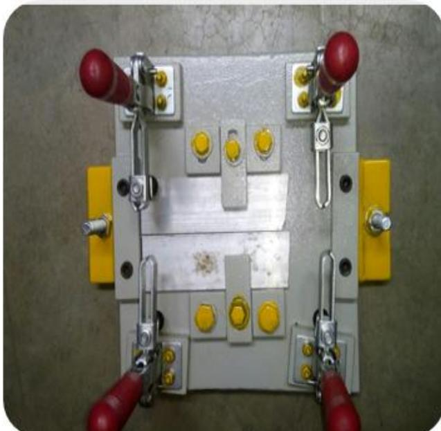
**Figure 6: Assembled fixture**
