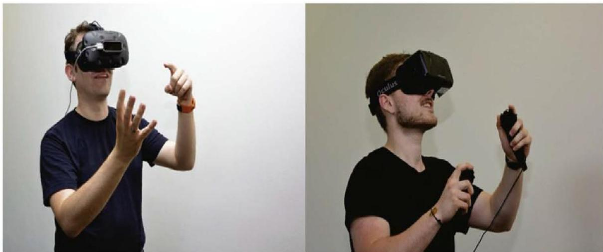
**Fig. 2 : Left- An HMD called HTC Vive as visual stereo display and a leap motion controller for tracking the hands; right- An HMD called Oculus Rift DK2 and a Razer Hydra controller for interaction.**
