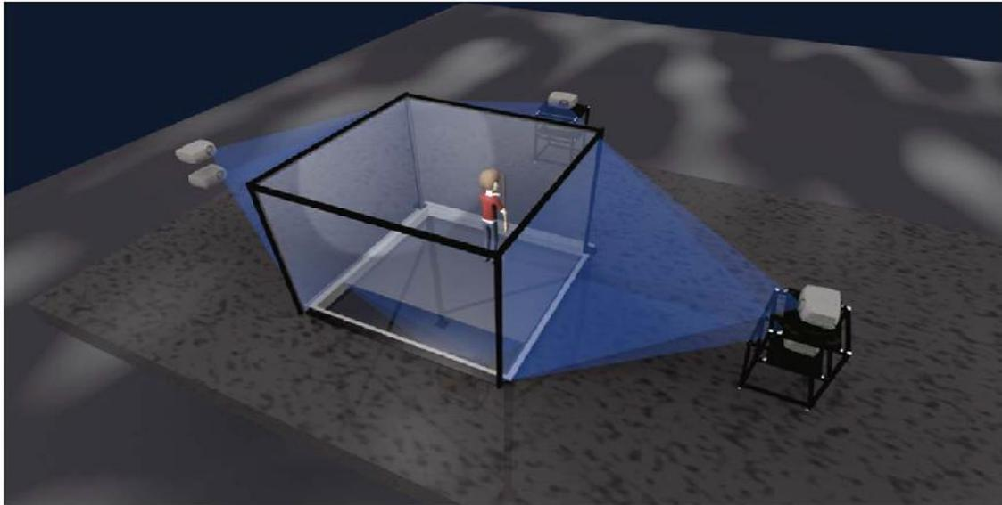
**Fig. 1: Three sides of a CAVE projected from the rear. The user's perspective is tracked using optical tracking systems.**
