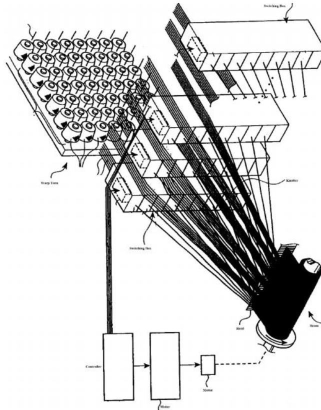
**Fig. 1 Arrangement of switching creel (Hiroshi & Shozo, 2007 )**
