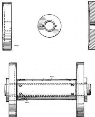
**Fig. 3 Warp knitting beam- Detailed view (Storey, 1965)**
