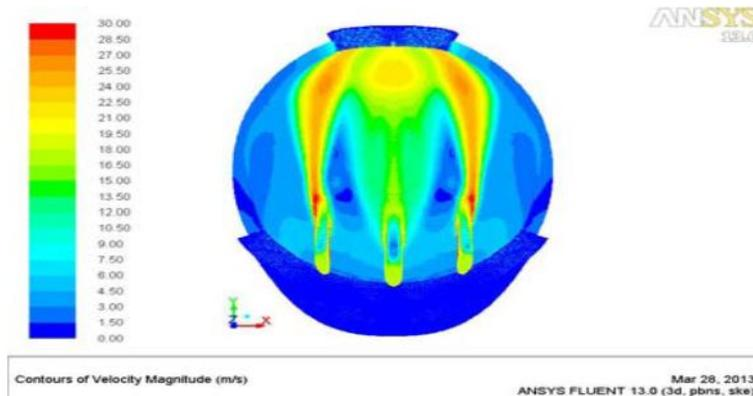
Fig. 4.4 velocity contour without exhaust fan
