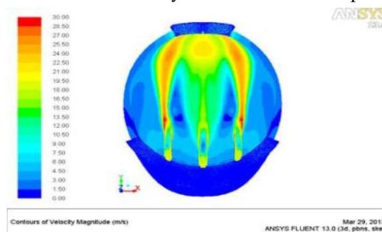
Fig.4.5 velocity contour with exhaust fan
