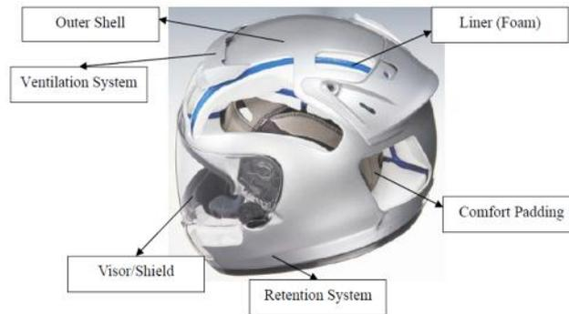
Fig.4.1 Components of a helmet
