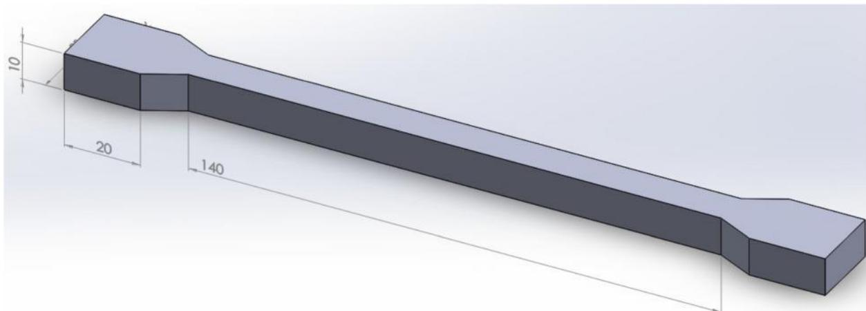
**Fig. 9: tensile specimen sample**
