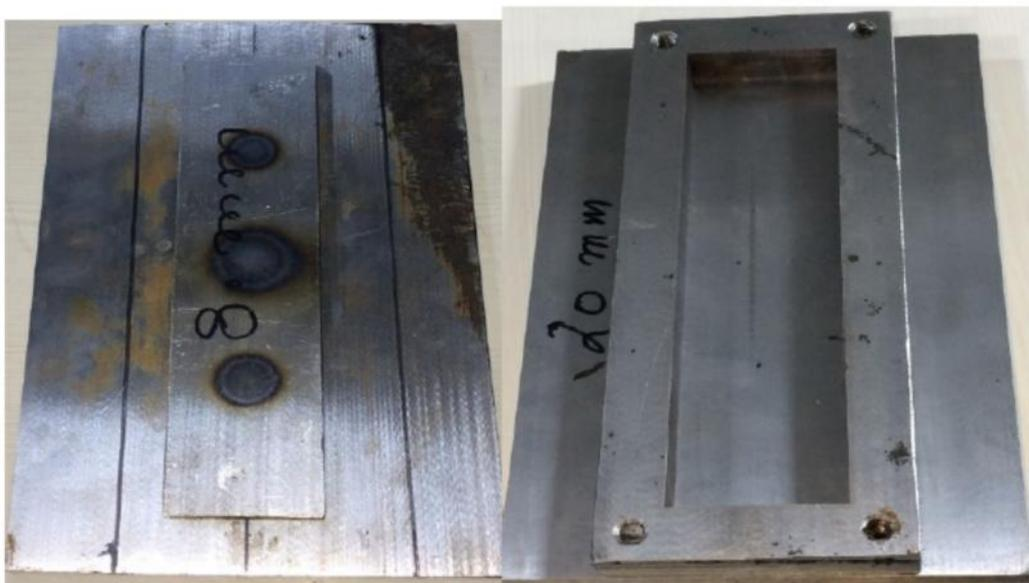
Fig. 4(a) fabricated mold parts
