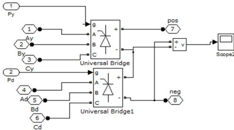
**Fig. 8: Double Bridge thyristor-controlled AC-DC converter**
