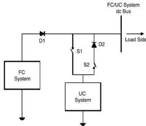
**Fig. 9: FC-UC hybrid system**
