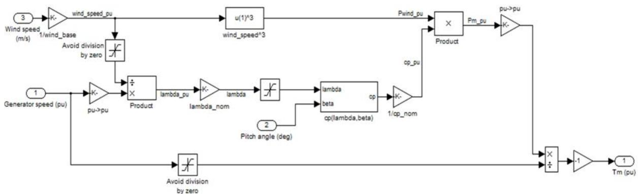
**Fig. 2: Simulink model of wind turbine**
