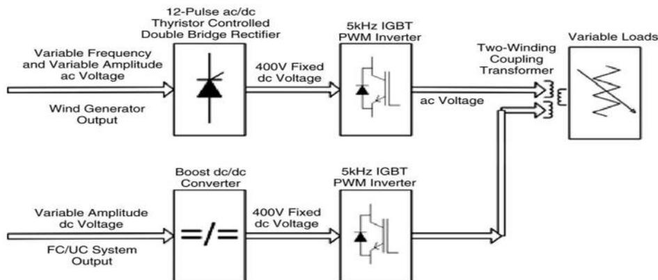
**Fig. 7: power controllers of the system bus**
