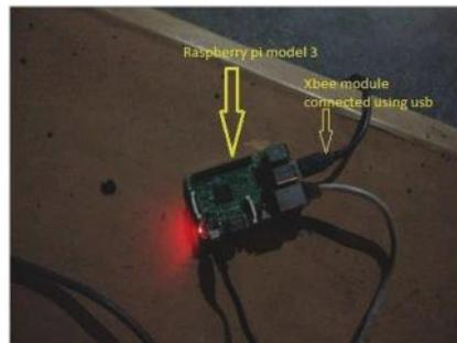
Fig. 8 Raspberry Pi module is connected to Xbee module
