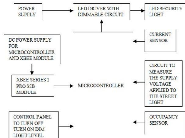
Fig: 3 Block diagram of Luminaire (Router) side
