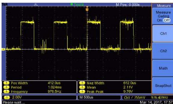
Fig.5 Microcontroller PWM output
