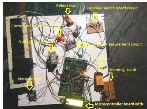
Fig. 4 Diagram of Microcontroller unit with circuits for different sensors before installation at luminaire
