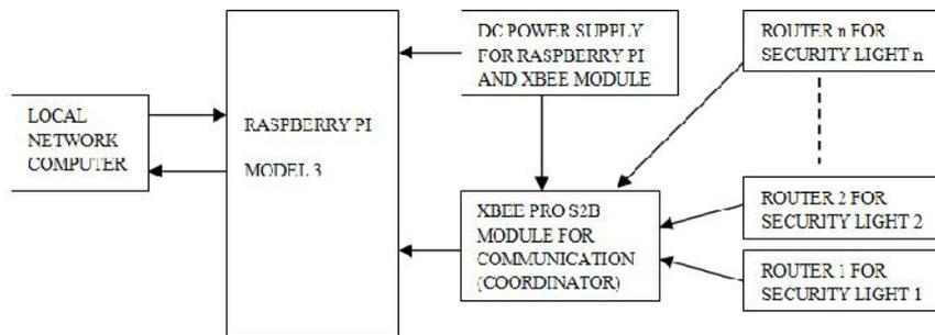
Fig.2 Block Diagram of the Local control unit side (Coordinator)
