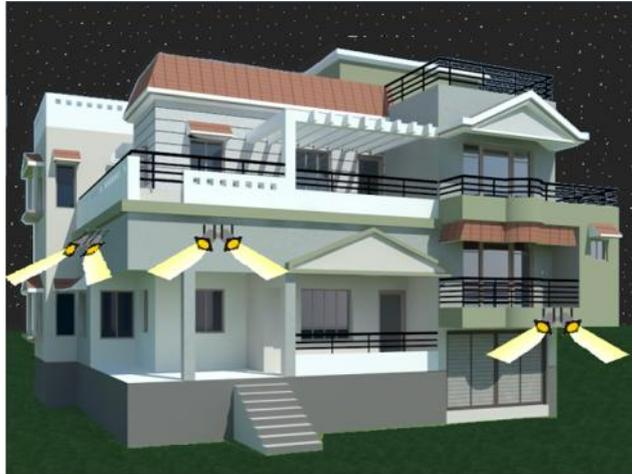
Fig. 1 Location of security lights around a building premise
