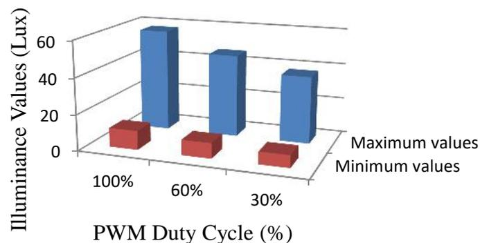
Fig. 10 Bar graph of the luminaire illuminance max & min values at different PWM duty cycle values
