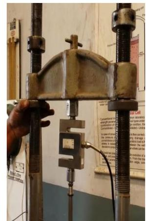
**Fig. 3b** Triaxial loading arrangement with 'S' type load cell
