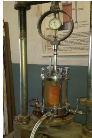
**Fig. 3a** Triaxial loading arrangement with proving ring
