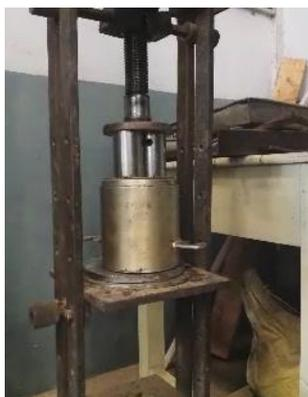
**Fig. 2a** Mechanically driven jack
