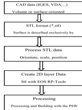
Fig 10: Sequence for Data preparation.
