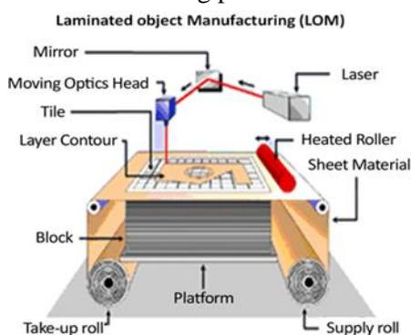
**Fig 2: The Schematic Diagram of LOM**
