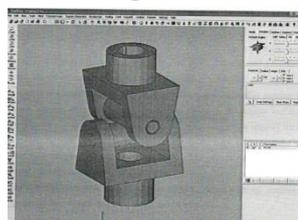
**Fig 16: STL file loaded at an orientation of 90° in Magics RP**
