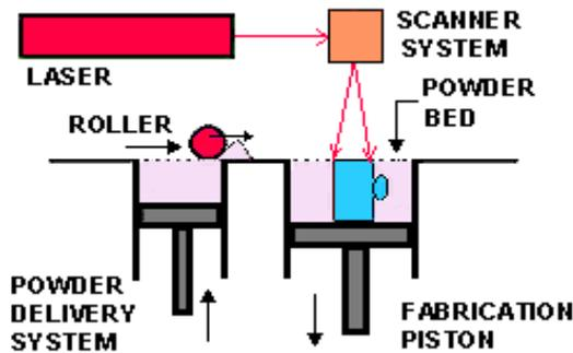
Fig 7: The Schematic Diagram of SLS
