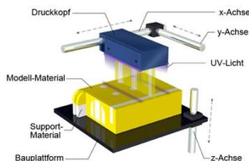
**Fig 5: Schematic Diagram of Multi jet modeling system**
