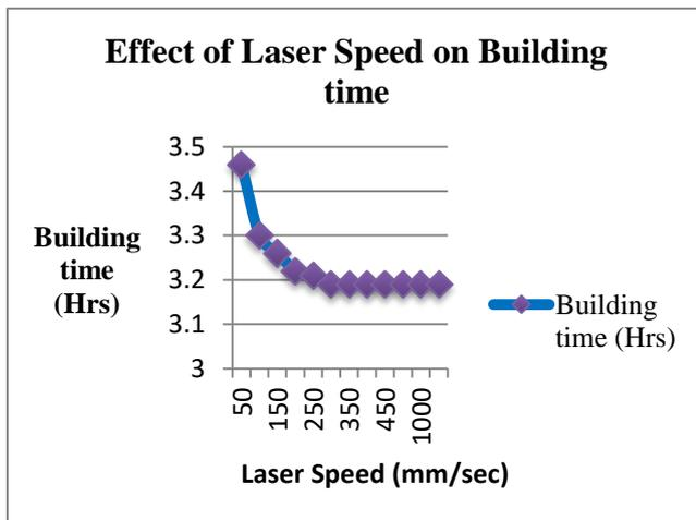
**Fig18: Effect of Laser speed on building time**
