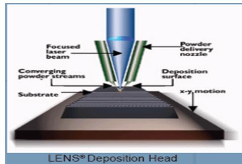
**Fig 6: The Schematic Diagram of LENS.**
