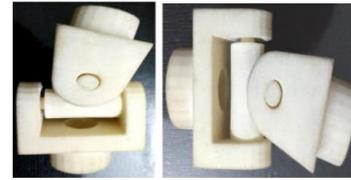
Fig 9: Hooke’s Joint by using the EOS RP-Tools
