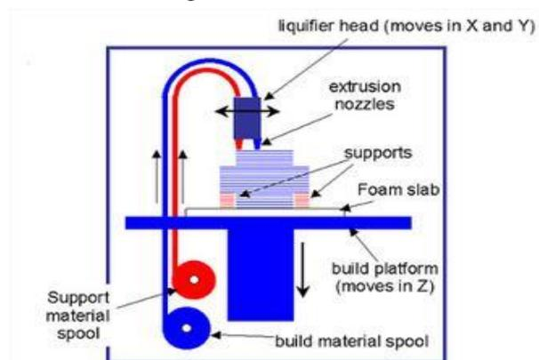
**Fig 3: The Schematic Diagram of FDM**
