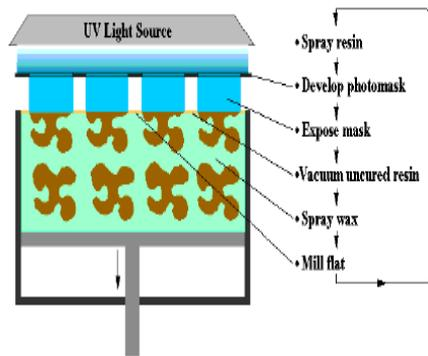
**Fig 4: Schematic Diagram of Solid Ground Curing**
