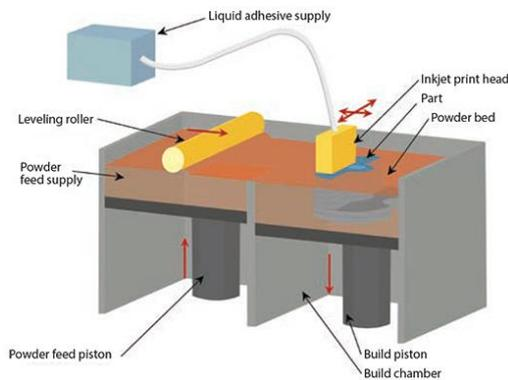
Fig 8: The Schematic Diagram of 3-DP.
