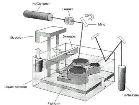
**Fig 1: Schematic Diagram of SLA Process**
