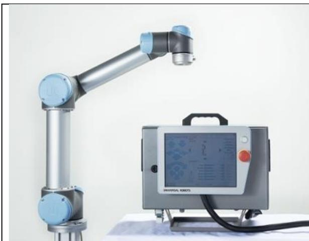
Fig.7 Typical Cobotic System
