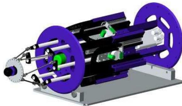
**fig 5 : 6 DOF Haptic robot**
