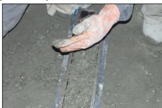
Figure 1.5 – Filling of moulds with concrete mixed with bacteria
