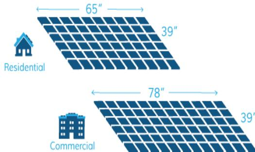
Fig. 2. Comparison of solar panel size [13]
