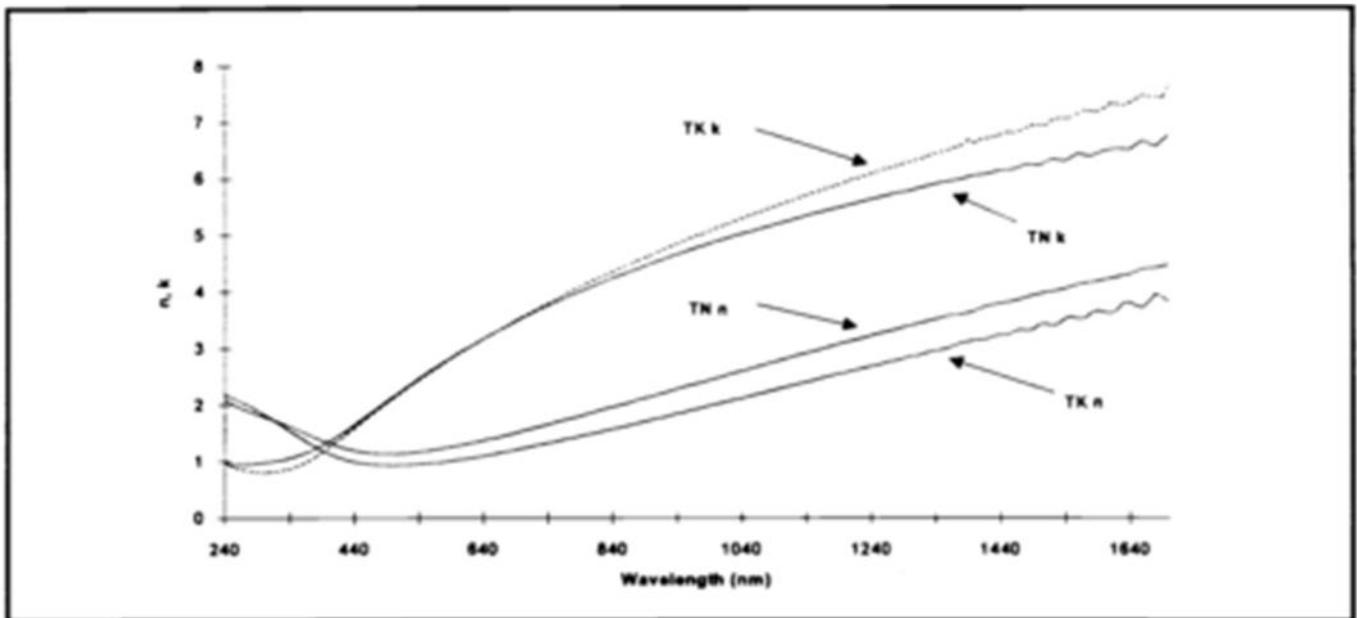
*Figure 2 optical constant TK and TN, VASE measured HfN*
