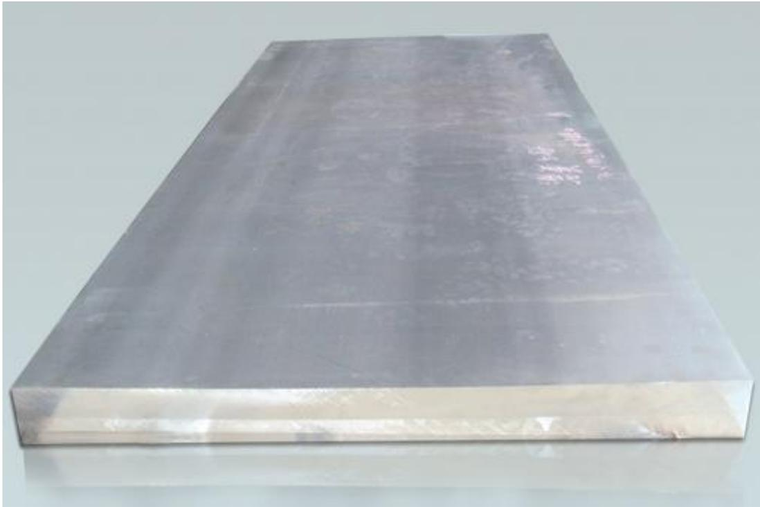
Fig 2.1 Aluminium plate AA6063
