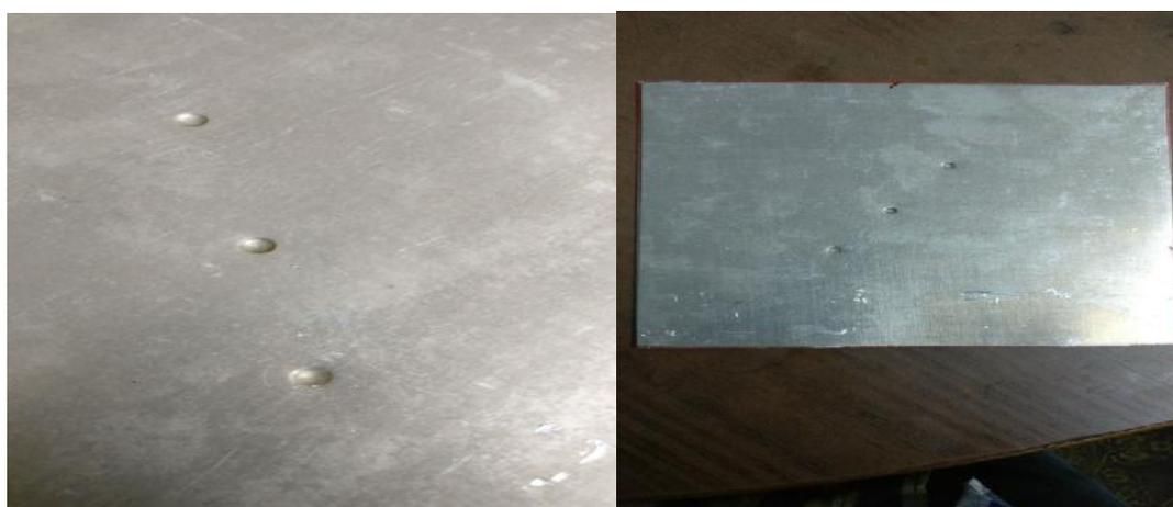
Fig 3.1 Brinell hardness indentation before FSP
