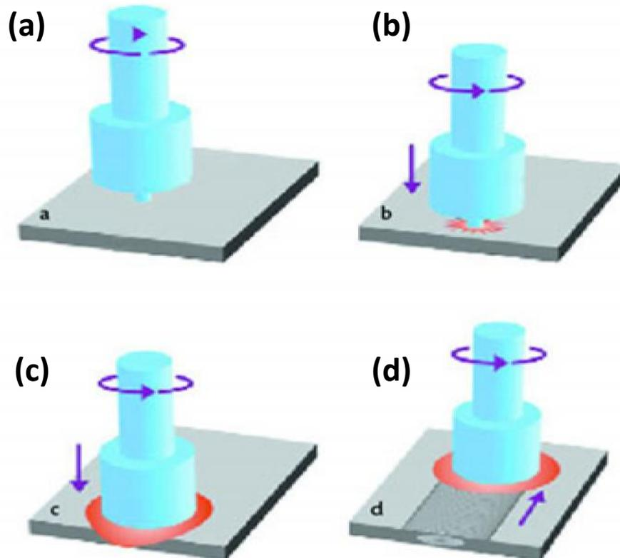
Fig. 1.1. Schematic illustration of friction stir processing: (a) rotating tool prior to contact with the plate; (b) tool pin makes contact with the plate, creating heat; (c) shoulder makes contact, restricting further penetration while expanding the hot zone; and (d) plate moves relative to the rotating tool, creating a fully recrystallized, fine grain microstructure.
