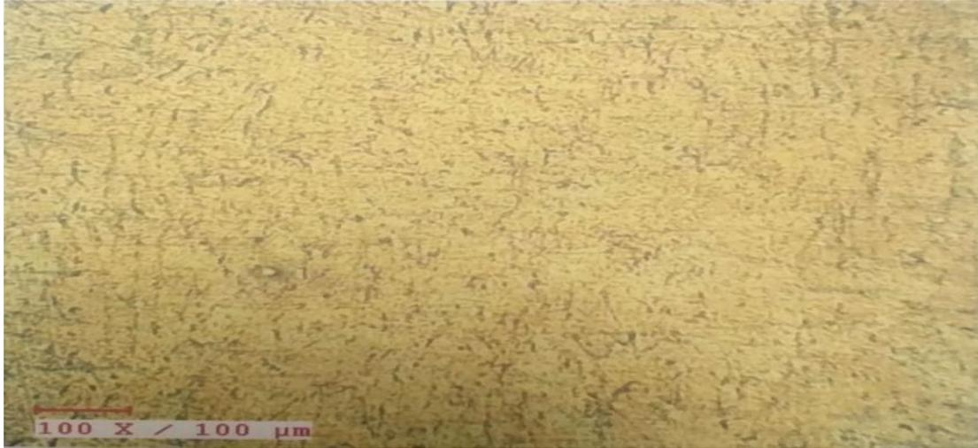
Fig 3.4 Microstructure of Al plate after FSP
