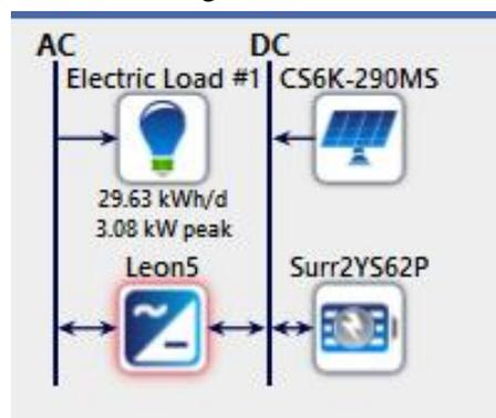
Fig.4 Configuration of PV-Battery System.
