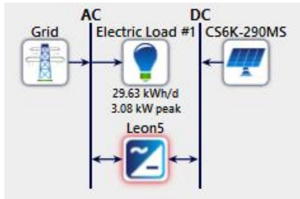
Fig.3 Configuration of PV-Grid System.
