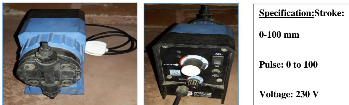
Figure.4: Dosing Injection pump
