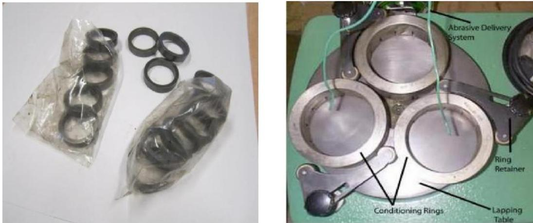
Figure 1: Stainless Steel Work piece
