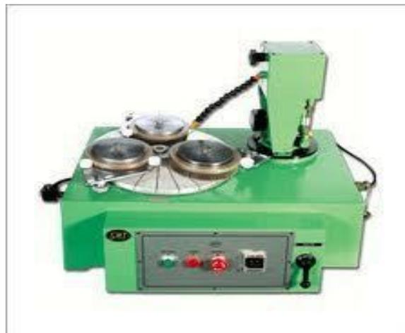
Figure 2: Single Plate lapping machine
