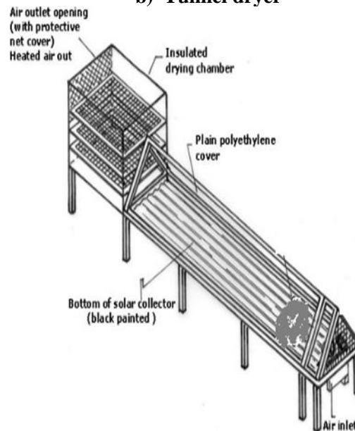
**Fig 5: Tunnel type indirect dryer[60]**
