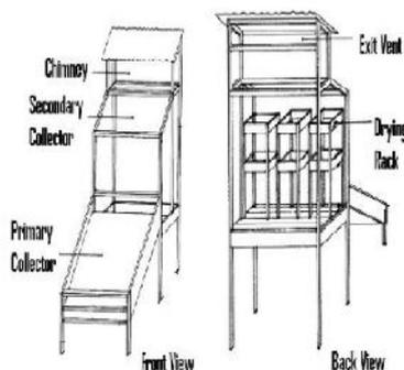
**Fig 6: Cabinet type mixed mode dryer [25]**
