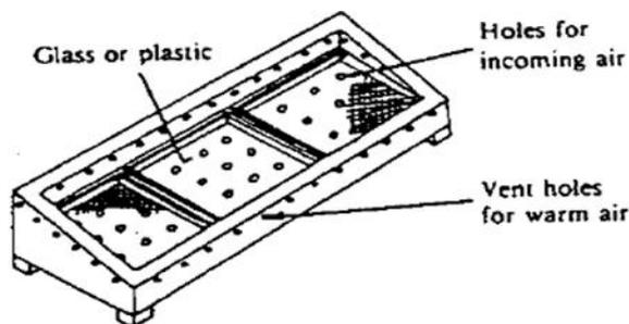
**Fig 2: Box type solar dryer [52]**
