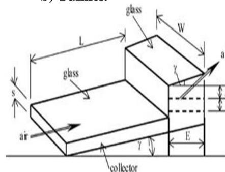
**Fig 7: Tunnel type mixed mode dryer[61]**
