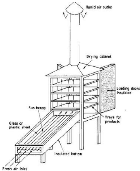
**Fig 4: Cabinet type indirect dryer[52]**
