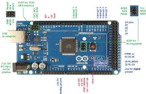
The Arduino Mega 2560 is a microcontroller board based on the ATmega2560. It has 54 digital input/output pins (of which 15 can be used as PWM outputs), 16 analog inputs, 4 UARTs (hardware serial ports), a 16 MHz crystal oscillator, a USB connection, a power jack, an ICSP header, and a reset button. It contains everything needed to support the microcontroller; simply connect it to a computer with a USB cable or power it with a AC-to-DC adapter or battery to get started.
