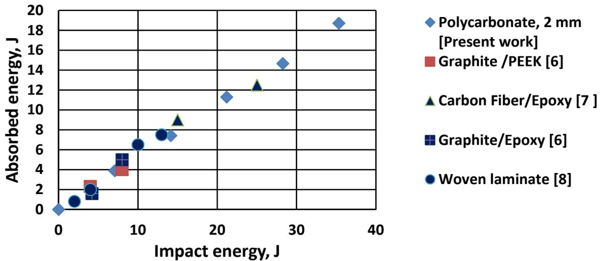
Figure 11 : Absorbed energy vs Impact energy for Polymeric materials
