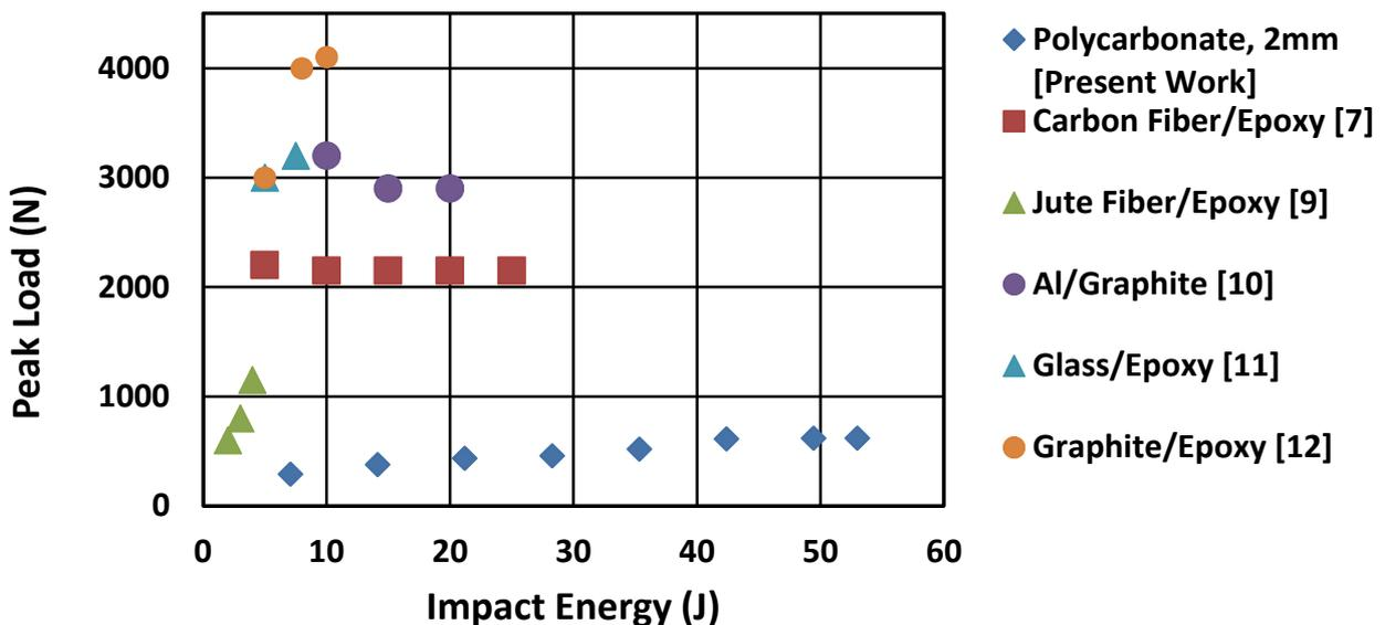
Figure 12 : Peak load versus Impact energy for different polymeric materials
