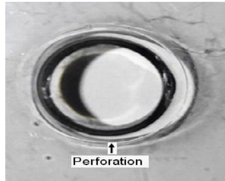
Figure 9: Force – time plot and indentation damage (Specimen: A-LVI-08).
