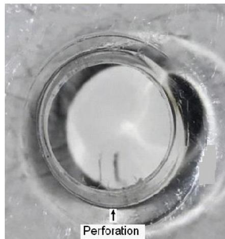
Figure 7: Force – time plot and indentation damage (Specimen: A-LVI-06).
