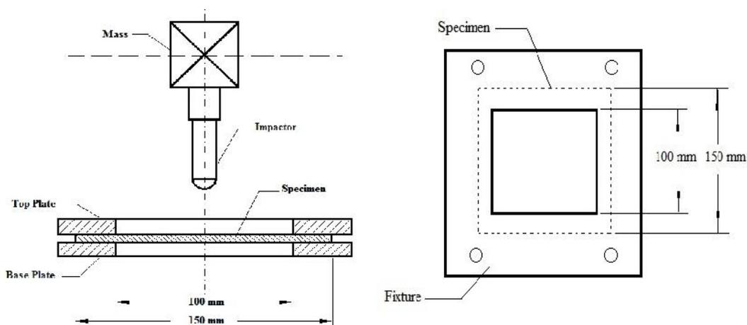
Figure 1 : Schematic of the low velocity drop-weight impact test
