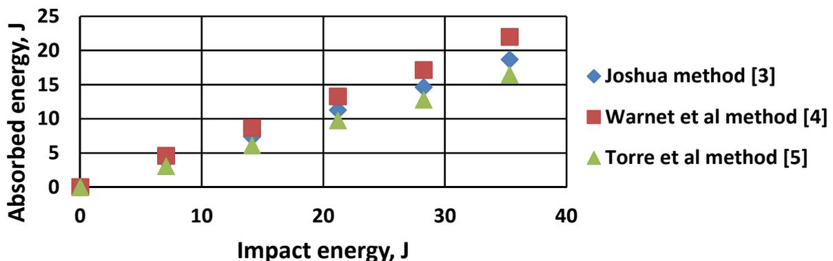
Figure 10 : Impact energy versus absorbed energy of Polycarbonate sheet
