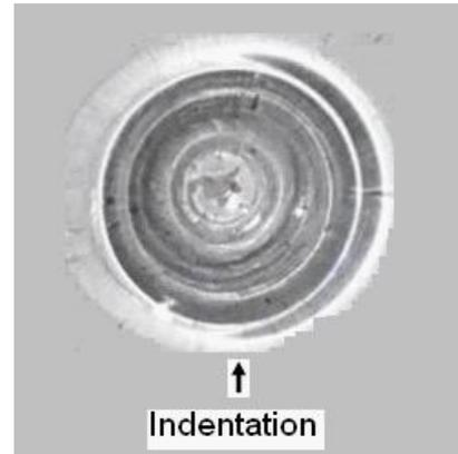
Figure 3: Force – time plot and indentation damage (Specimen: A-LVI-02).
