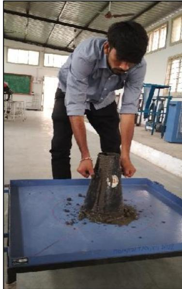
**Figure 4 - Slump testing**
